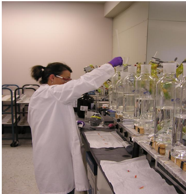
Jennifer Ratliff (Pesticide/PCB Section) changes over the pH on some groundwater samples being prepared for (ABN) semi-volatile analysis.
