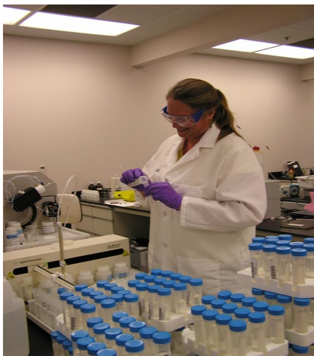
JoEllen Thompson (Metals Section) loads the autosampler on an Inductively Coupled Plasma Mass Spectrometer (ICPMS) instrument with DOW water samples for analysis.
