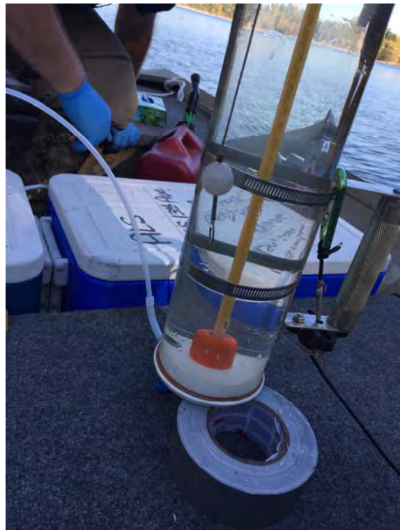
Photo 2: Tubing to transfer surface water from the sampler to the sampling containers.
