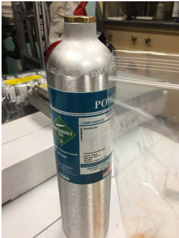
Photo 7: Inert argon gas, unlike helium or nitrogen, is heavier than air and will fill up the bag, used to enclose the peeper for sample transfer, from the bottom first, including the containers.
