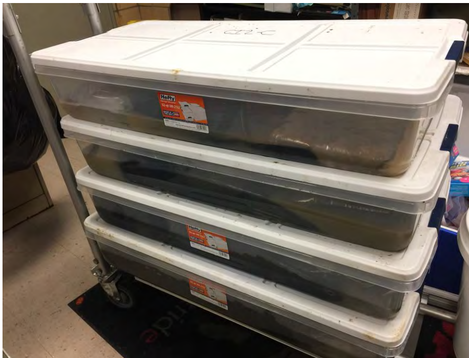
Photo 4: Multiple passive diffusion peeper pore water samples, retained in their native sediment prior to pore water extraction.
