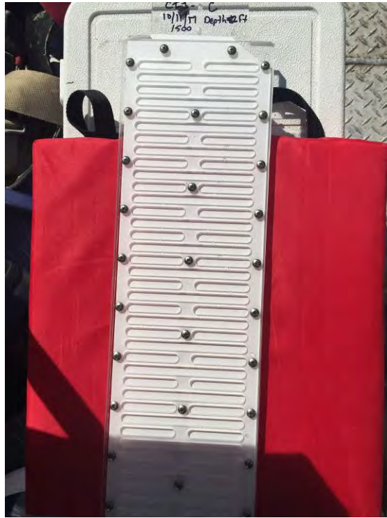
Photo 1: A new passive diffusion pore water "peeper" ready for deployment on the dive boat.
