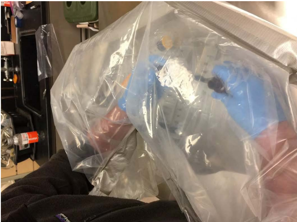
Photo 9: Maintaining an anoxic environment while transferring the pore water from the hypodermic needle(s) into the appropriate containers.
