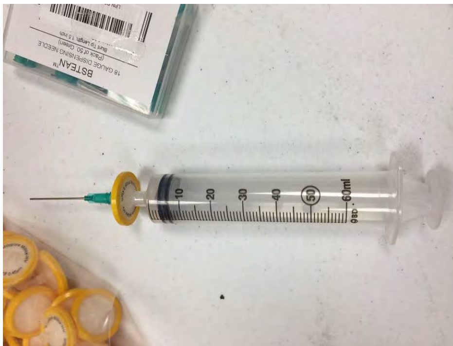
Photo 6: Sterile (one-time use) 60ml hypodermic needle and 0.45um filter for extracting filtered pore water from a peeper.
