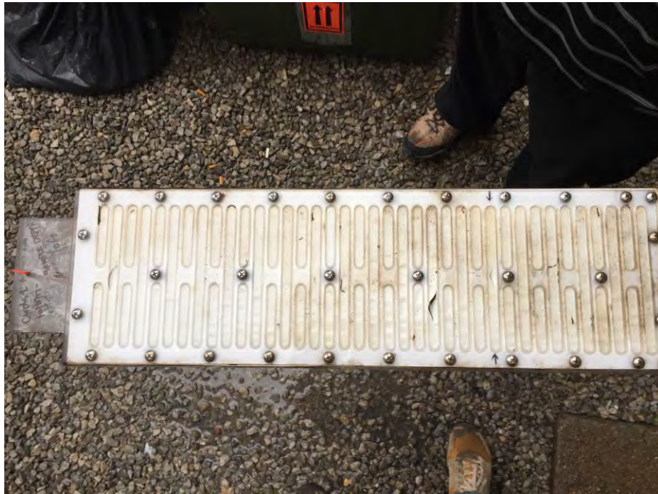
Photo 5: A retrieved peeper prior to pore water extraction.
