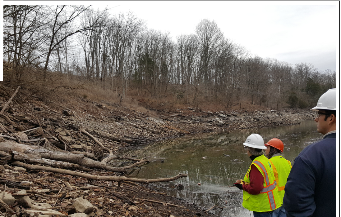
2. January 19, 2017, Lake elevation 729 feet with no visible evidence of springs or potential groundwater migration to Curds Inlet in an area of Curds Inlet near the coal pile.
