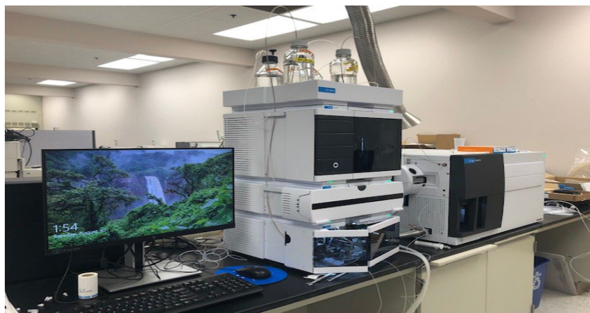
Agilent 6470A Triple Quadrupole LC/MS
