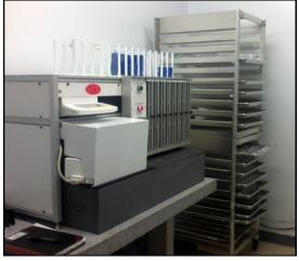
The TSB's particulate weigh lab contains a robotic device called an "autohandler," which is used to weigh  $\text{PM}_{2.5}$  and  $\text{PM}_{10}$  filters.
