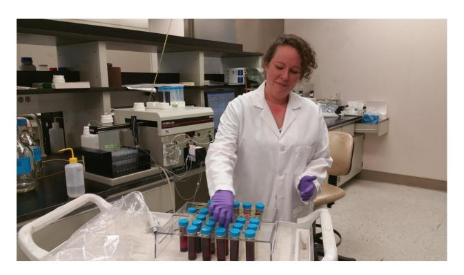
Amanda Evans (Metals Section) loads DOW water mercury samples on a Leeman Hydra AA instrument.
