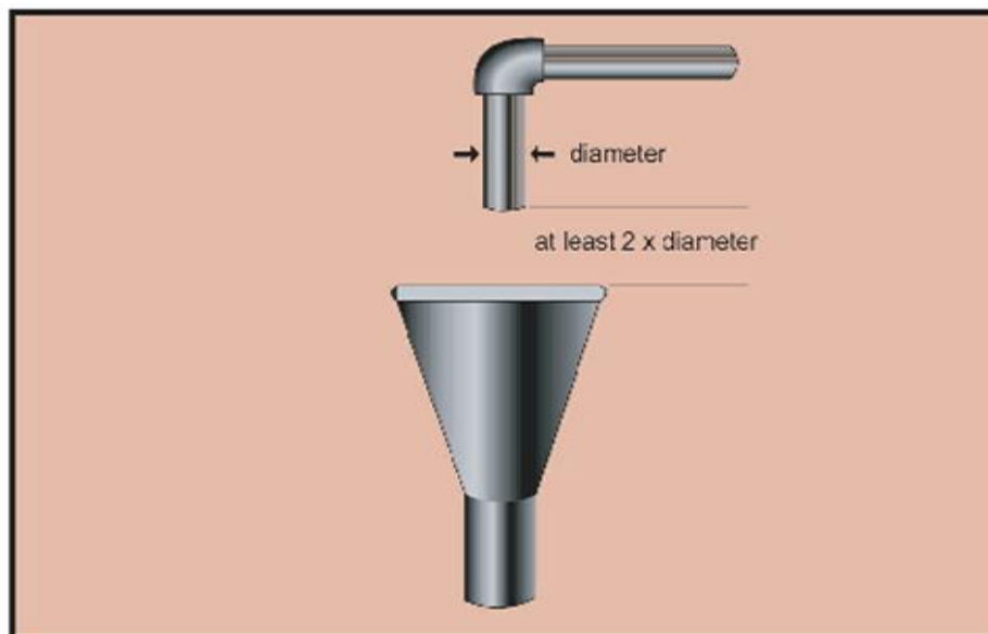
8.4.1 Figure 1: Air gap
