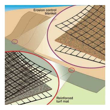
Erosion control blankets are thinner and usually degrade quicker than turf reinforcement mats. Check manufacturer's product information for degradation rate (life span), slope limitations, and installation. Remember to apply seed, fertilizer, and lime before covering with blankets or mats!
