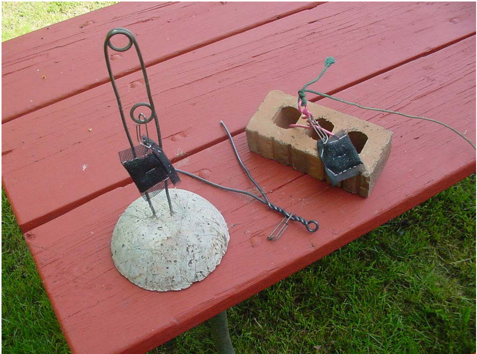
Figure 8: Activated charcoal packet dye receptors attached by trot-line clip to “Quinlan Gumdrops” or brick fitted with #10 copper wire. Devices secured to retrieval point with nylon cord.
