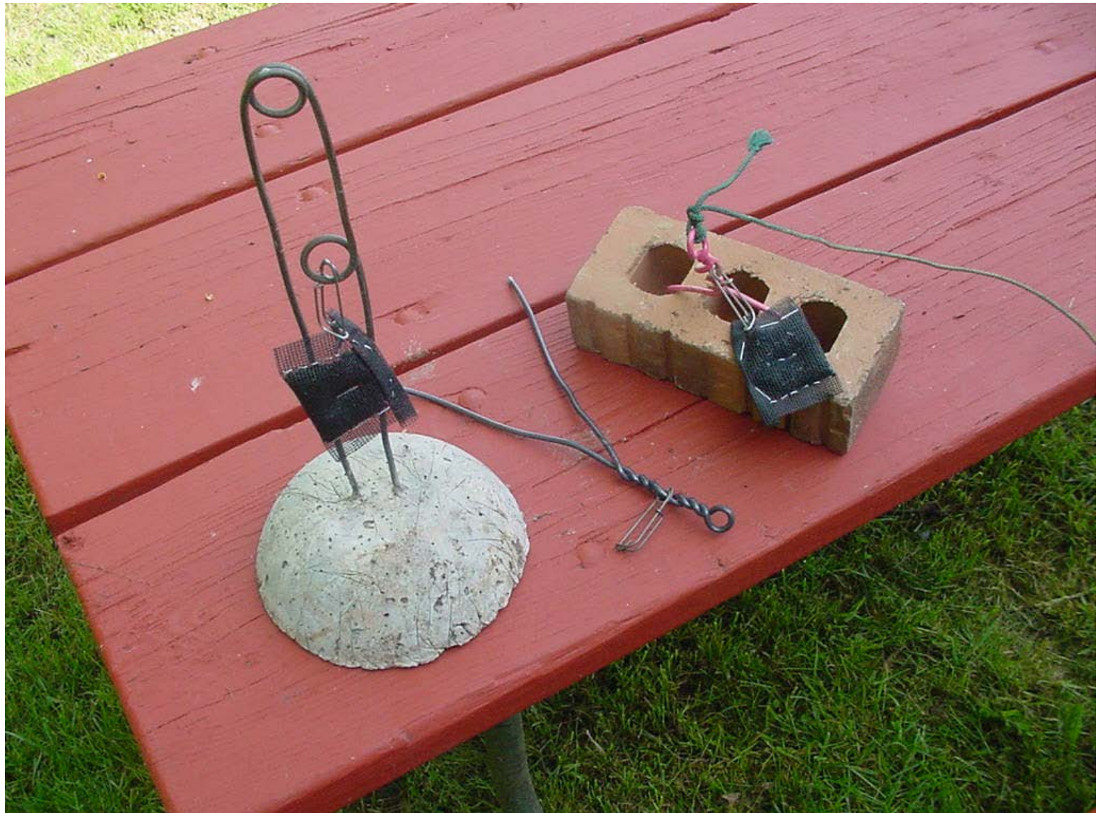
Figure 5. Activated charcoal packet attached by trot-line clip to “Quinlan Gumdrop” or brick fitted with #10 copper wire. Devices secured to retrieval point with nylon cord.
