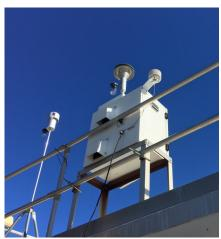
Particulate matter sampler. (Photo: DAQ)
