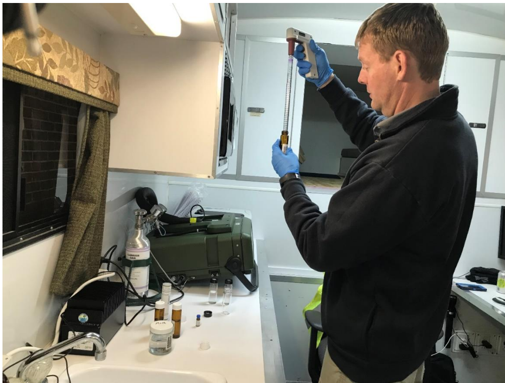
Photo 24: Staff Conducting Monitoring Using a Mobile GC/MS. Photo by Robert Francis.
