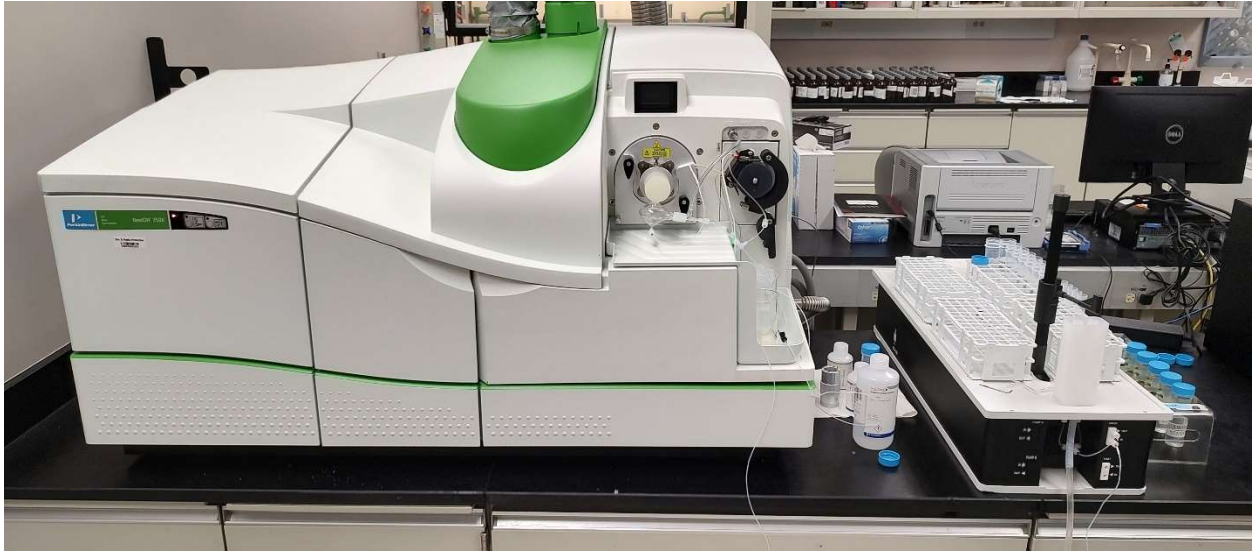
NexION 350 ICP-MS used for the analysis of WIIN Grant Samples
