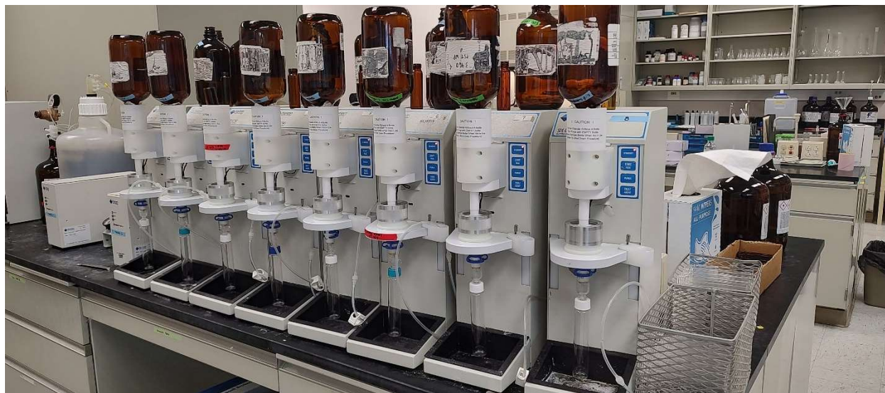
Horizon Solid Phase Extractors used for the extraction of organic compounds from liquid samples.
