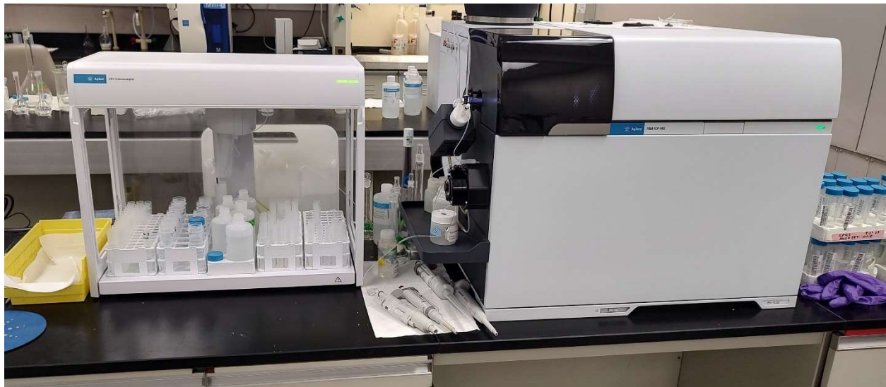
ICP-MS (Inductively Coupled Plasma – Mass Spectrometer) used for metals analysis
