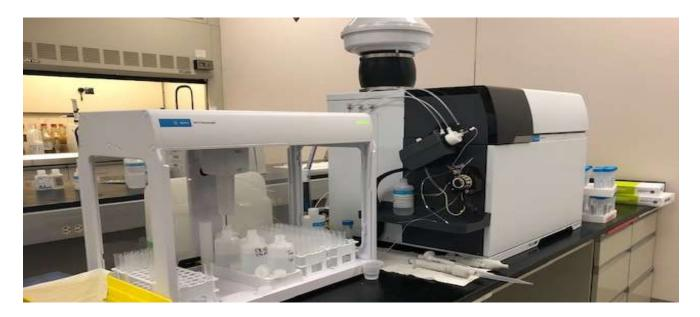
The lab was also able to acquire enough funding to purchase a new Discrete Analyzer (DA) in the Standard Testing Section. This is the fourth DA that the lab has purchased since 2010. This instrument has already taken over the duties of one that is not able to be serviced. This was perfect timing and much needed in order for the lab to continue providing Ammonia, Sulfate and Nitrate testing for the department.
