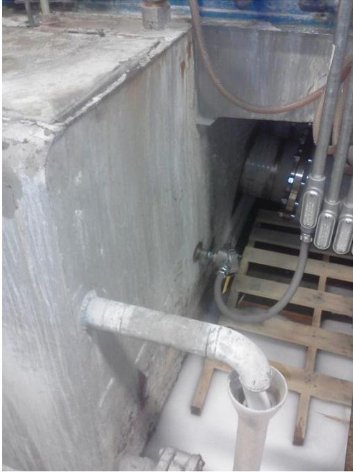
The picture to the left is an example of an electric immersion heater placed into a process tank that replaces the use of steam in a paint process.
