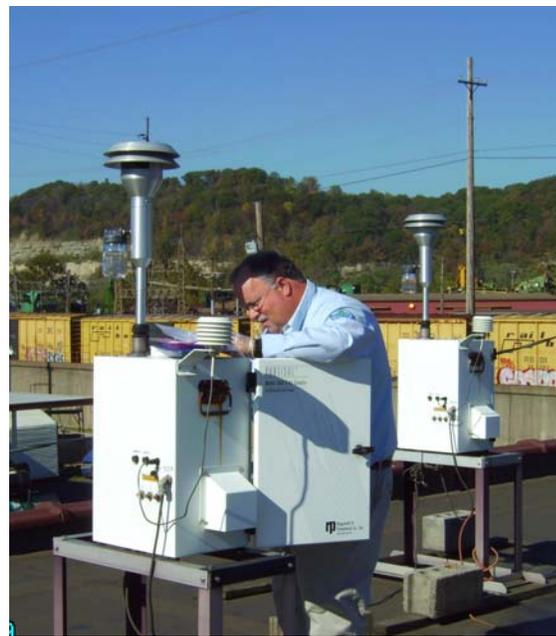
***Air monitors are located at monitoring stations or on building rooftops as seen in the left and right pictures. The center picture is a particulate matter monitor used by DAQ to speciate  $\text{PM}_{2.5}$ .***
