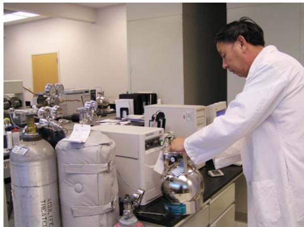
Kassandra Rumsey prepares mercury samples for analysis and Baoding Chen prepares a SUMMA canister for an air analysis.
