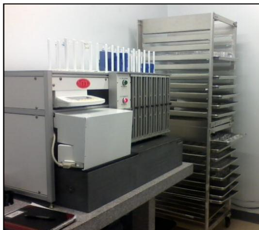
The TSB's particulate weigh lab contains a robotic device called an "autohandler," which is used to weigh PM<sub>2.5</sub> and PM<sub>10</sub> filters.
