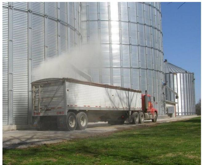
Fugitive emissions from grain loading. State regulation requires control measures to reduce fugitive emissions and their impact on air quality.
