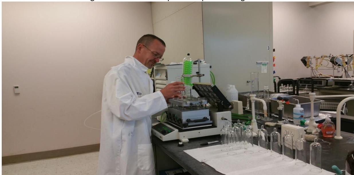
Eric Scott (Technical Services Section Supervisor) loads samples onto the Buchi Syncore Evaporator.
