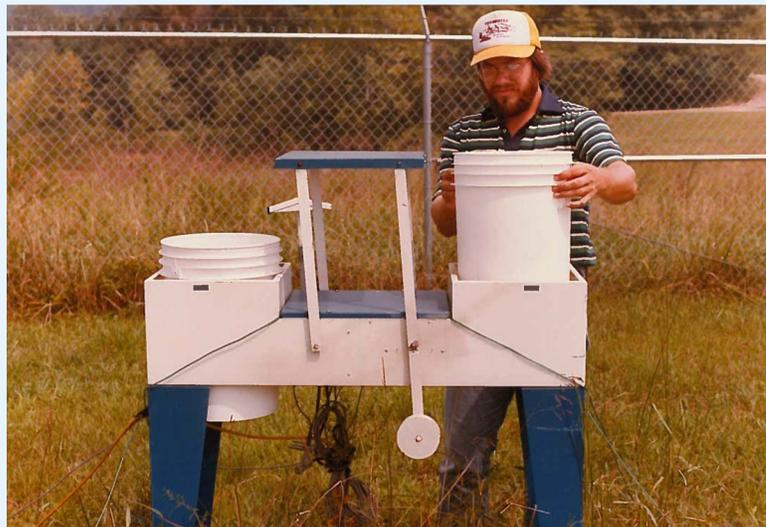
This photo taken in the 1980's shows DAQ scientist George Hockley working with an acid precipitation collector. Photo: DAQ
