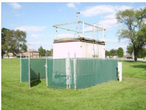
The monitoring site is a stationary equipment shelter located on the grounds of the Oakland Elementary School in Oakland, Kentucky. The sample inlets are 61 meters from the nearest road. The most recent site inspection was conducted on December 17, 2009. Upon inspection, the sample inlets and monitors were found to be in good condition. The site meets the requirements of 40 CFR 58, Appendices C, D, E and G.
