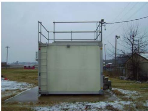
The monitoring site is a stationary equipment shelter located on the grounds of the KY DOT Highway Garage in Smithland, Kentucky. The sample inlets are 143 meters from the nearest road. The most recent site inspection was conducted on December 17, 2009. Upon inspection, the sample lines and monitors were found to be in good condition. The site meets the requirements of 40 CFR 58, Appendices C, D, E and G.
