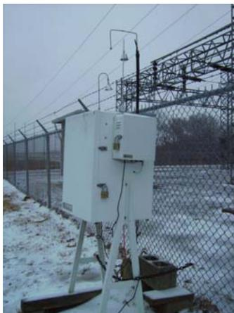
The monitoring site is an air toxics monitor location off Ballpark Road in Calvert City, Kentucky. The sample inlets are 2 meters above ground level. The inlets are 65 meters from the nearest road. The most recent site inspection was conducted on December 17, 2009. Upon inspection, the sample inlets and monitors were found to be in good condition.
