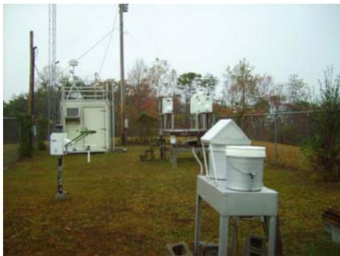
The monitoring site is a stationary equipment shelter in a fenced area located in a remote section of Camp Webb in Grayson, Kentucky. The nearest road is a service road to the site and is 98 meters from the site. The most recent site inspection was conducted on December 28, 2009. Upon inspection, the sample lines and monitors were found to be in good condition. The site meets the requirements of 40 CFR 58, Appendices C, D, E and G.
