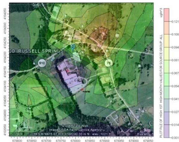
Superior Battery, located in Russell Springs, Kentucky, was identified as a lead source emitting over 1 tons per year of actual reported emissions in 2006. In accordance with 40 CFR Part 58 Appendix D, a lead source monitoring site will be located at the Salem Elementary School in Russell Springs, Kentucky. The location of this source-oriented lead monitor was determined through the use of AERMOD modeling analysis.
