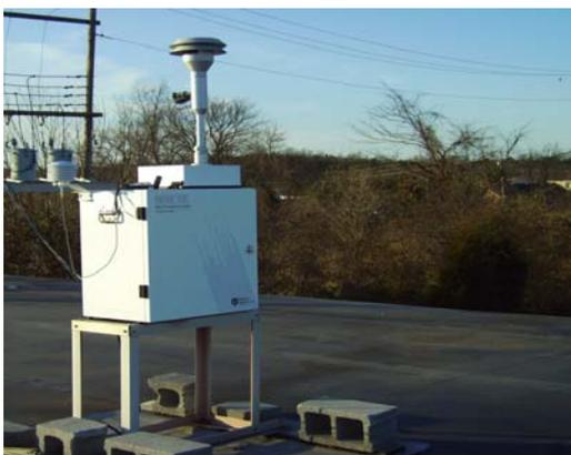
The monitoring site is located on the roof of the Ragland Building in Frankfort, Kentucky. The sample inlet is 138 meters from the nearest road. The most recent site inspection was conducted on November 25, 2009. Upon inspection, the sample inlet and monitor were found to be in good condition. The site meets the requirements of 40 CFR 58, Appendices C, D and E.
