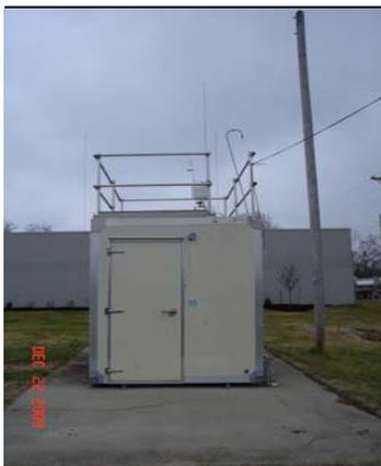
The monitoring site is a stationary equipment shelter located on the grounds of the Firearms Training Center in Louisville, Kentucky. The sample inlet is 4 meters above ground level and 49 meters from the nearest road. The most recent site inspection was conducted on December 21, 2009. The air monitoring site was found to be in accordance with 40 CFR Part 58, Appendices C, D, E and G.
