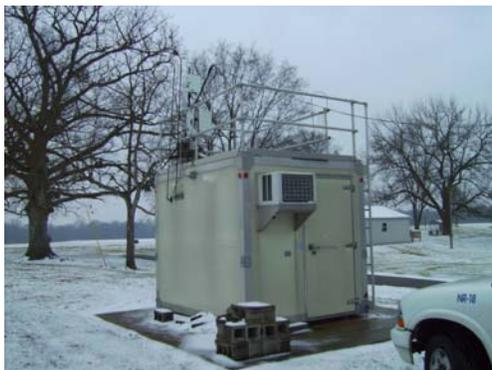
The monitoring site is a stationary equipment shelter located at the residence of 763 Bloodworth Road in Livingston County, Kentucky. The sample inlets are 8 meters from the nearest road. The most recent site inspection was conducted on December 17, 2009. Upon inspection, the sample lines and samplers were found to be in good condition.
