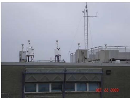
The monitoring site is located on the roof of the Southwick Community Center in Louisville, Kentucky. The sample inlets are 6 meters above ground level and 45 meters from the nearest road. The most recent site inspection was conducted on December 21, 2009. The air monitoring site was found to be in accordance with 40 CFR Part 58, Appendices C, D, E and G.
