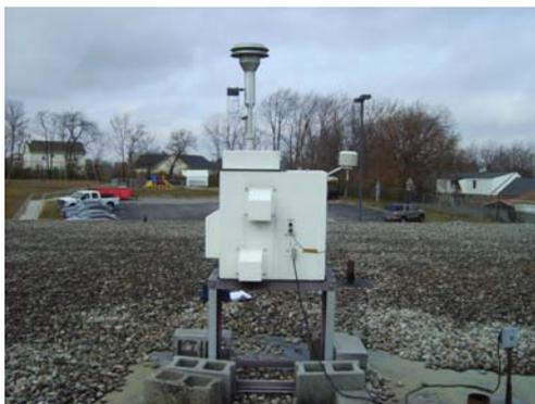
The monitoring site is located on the roof of the Mayfield Elementary School in Richmond, Kentucky. The sample inlets are 72 meters from the nearest road. The most recent site inspection was conducted on November 5, 2009. Upon inspection, the sample inlet and monitor were found to be in good condition. The site meets the requirements of 40 CFR 58, Appendices C, D and E.
