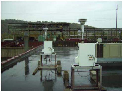
The monitoring site is located on the west end of the roof of the Ashland Valvoline Oil complex building in Ashland, Kentucky. The building is one story tall. The sample inlets are 30 meters from the nearest road. The most recent site inspection was conducted on December 28, 2009. Upon inspection, the sample inlets and monitors were found to be in good condition. The site meets the requirements of 40 CFR 58, Appendices C, D and E.
