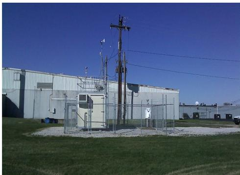
The monitoring site is a stationary equipment shelter located on the grounds behind the Wyndall's Shopping Center in Owensboro, Kentucky. The sample inlets are 46 meters from the nearest road. The most recent site inspection was conducted on November 10, 2009. Upon inspection, the sample lines and monitors were found to be in good condition. The site meets the requirements of 40 CFR 58, Appendices C, D, E and G.
