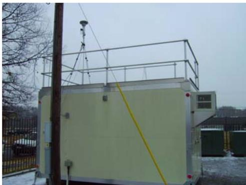
The monitoring site is a stationary equipment shelter located on the grounds of the Jackson Purchase RECC in Paducah, Kentucky. The sample inlets are 10 meters from the nearest road. The most recent site inspection was conducted on December 17, 2009. Upon inspection, the sample inlets and monitors were found to be in good condition. The site meets the requirements of 40 CFR 58, Appendices C, D, E and G.
