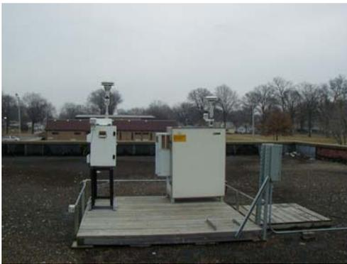
The monitoring site is located on the roof of the recreation building at Wyandotte Park in Louisville, Kentucky. The sample inlets are 5 meters above ground level and 54 meters from the nearest road. The most recent site inspection was conducted on December 21, 2009. The air monitoring site was found to be in accordance with 40 CFR Part 58, Appendices C, D, E and G.
