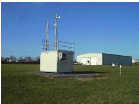
The monitoring site is a stationary equipment shelter located on the grounds of the Kentucky DOT Garage in Nicholasville, Kentucky. The sample inlets are 113 meters from the nearest road. The most recent site inspection was conducted on November 5, 2009. Upon inspection, the sample inlets and monitors were found to be in good condition. The site meets the requirements of 40 CFR 58, Appendices C, D, E and G.
