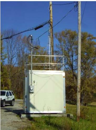
The monitoring site is a stationary equipment shelter located at the intersection of KY 338 and Lower River Road in East Bend, Kentucky. The sample inlets are 15 meters from the nearest road. The most recent site inspection was conducted on November 4, 2009. Upon inspection, the sample lines and monitors were found to be in good condition. The site meets the requirements of 40 CFR 58, Appendices C, D and E.
