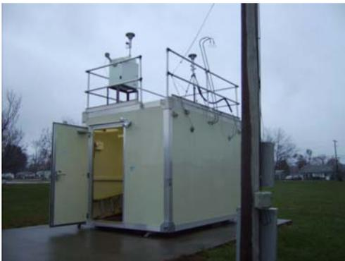
The monitoring site is a stationary equipment shelter located on the grounds of the Watson Lane Elementary School in Louisville, Kentucky. The sample inlets are 4 meters above ground level and 30 meters from the nearest road. The most recent site inspection was conducted on December 21, 2009. The air monitoring site was found to be in accordance with 40 CFR Part 58, Appendices C, D, E and G.
