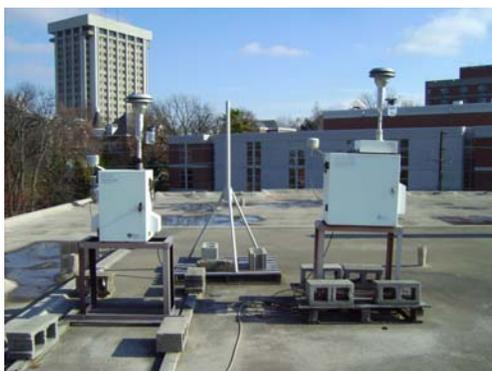
The monitoring site is located on the roof of the Whalen Transportation Research Building on the University of Kentucky campus in Lexington, Kentucky. The sample inlets are 18 meters from the nearest road. The most recent site inspection was conducted on November 5, 2009. Upon inspection, the sample inlets and monitors were found to be in good condition. The site meets the requirements of 40 CFR 58, Appendices C, D and E.
