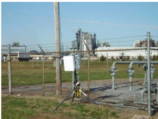
The monitoring site is an air toxics monitor location off KY95 in Calvert City, Kentucky. The sample inlet is 2 meters above ground level and 43 meters from the nearest road. The most recent site inspection was conducted on December 17, 2009. Upon inspection, the sample inlet and monitor were found to be in good condition.
