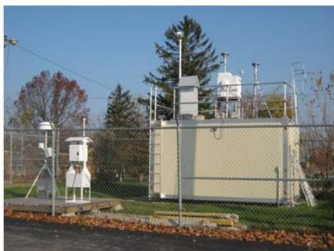
The monitoring site is a stationary equipment shelter located on the grounds of the Fayette County health department building in Lexington, Kentucky. The sample inlets are 117 meters from the nearest road. The most recent site inspection was conducted on November 5, 2009. Upon inspection, the sample lines and monitors were found to be in good condition. The site meets the requirements of 40 CFR 58, Appendices C, D, E and G.
