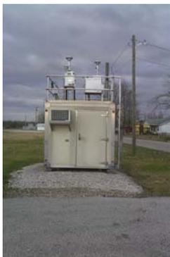
The monitoring site is a stationary equipment shelter located on the grounds of the Baskett Fire Department in Baskett, Kentucky. The sample inlets are 10 meters from the nearest road. The most recent site inspection was conducted on November 8, 2009. Upon inspection, the sample lines and monitors were found to be in good condition. The site meets the requirements of 40 CFR 58, Appendices C, D, E and G.
