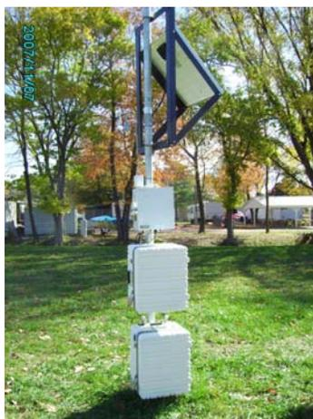
The monitoring site consists of a solar-powered, battery-charged air toxics monitor located on the Brady property of the Lazy Daz mobile home park, in Calvert City, Kentucky. The sample inlet is 154 meters from the nearest road. The most recent site inspection was conducted on December 17, 2009. Upon inspection, the sample inlet and monitor were found to be in good condition.
