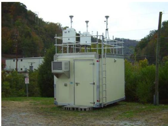
The monitoring site is a stationary equipment shelter located behind the DOT District Office building at 101 North Mayo Trail in Pikeville, KY. The sample inlets are 88 meters from the nearest road. The most recent site inspection was conducted on November 18, 2009. Upon inspection the sample lines and monitors were found to be in good condition. This site meets the requirements of 40 CFR 58, Appendices C, D, E and G.
