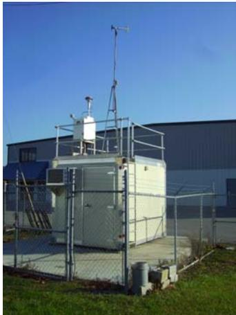
The monitoring site is a stationary equipment shelter located on the grounds of the Middlesboro Airport in Middlesboro, Kentucky. The sample inlets are 87 meters from the nearest road. The most recent site inspection was conducted on December 29, 2009. Upon inspection the sample lines and monitors were found to be in good condition. Even though this site is for special purpose monitoring, the site meets the requirements of 40 CFR 58, Appendices C, D, E and G.
