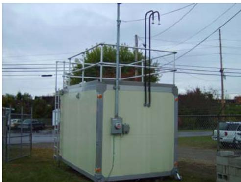
The monitoring site is a stationary equipment shelter located on the grounds of a water tower near the intersection of Scott Street and Center Avenue in Worthington, Kentucky. The sample inlets are 17 meters from the nearest road. The most recent site inspection was conducted on December 28, 2009. Upon inspection, the sample lines and monitors were found to be in good condition. The site meets the requirements of 40 CFR 58, Appendices C, D, E and G.
