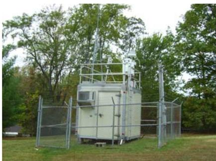
The monitoring site is a stationary equipment shelter located on the grounds of the health department building in Ashland, Kentucky. The sample inlets are 72 meters from the nearest road. The most recent site inspection was conducted on December 28, 2009. Upon inspection, the sample lines and monitors were found to be in good condition. The site meets the requirements of 40 CFR 58, Appendices C, D, E and G.
