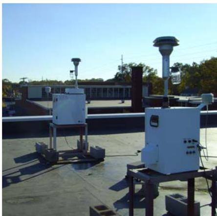
The monitoring site is located on the roof of the Paducah Middle School in Paducah, Kentucky. The sample inlets are 60 meters from the nearest road. The most recent site inspection was conducted on December 17, 2009. Upon inspection, the sample inlets and monitors were found to be in good condition. The site meets the requirements of 40 CFR 58, Appendices C, D and E.
