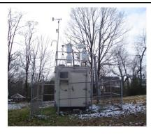
The monitoring site is a stationary equipment shelter located on the grounds of the health department building in Ashland, Kentucky. The sample inlets are 70 meters from the nearest road. Upon inspection, the sample lines and monitors were found to be in good condition. The site meets the requirements of 40 CFR 58, Appendices A, C, D, E and G.
