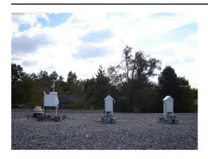
The monitoring site is located on the roof of the Mayfield Elementary School in Richmond, Kentucky. The sample inlets are 65 meters from the nearest road. Upon inspection, the sample inlet and monitor were found to be in good condition. The lead sampler is not located within the expected area of maximum deposition, as is required by 40 CFR 58, Appendix D. Otherwise, the site meets the requirements of 40 CFR 58, Appendices A, C, D and E.
