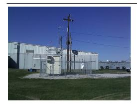
The monitoring site is a stationary equipment shelter located on the grounds behind the Wyndall's Shopping Center in Owensboro, Kentucky. The sample inlets are 48 meters from the nearest road. Upon inspection, the sample lines and monitors were found to be in good condition. The site meets the requirements of 40 CFR 58, Appendices C, D, E and G.
