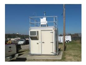
The monitoring site is a stationary equipment shelter located on the grounds of the Somerset Gas Company Warehouse on Clifty Street in Somerset, KY. The sample inlets are 10 meters from the nearest road, which is a dead-end street with little traffic. Upon inspection the sample line and monitors were found to be in good condition. The site meets the requirements of 40 CFR 58, Appendices C, D, and E.
