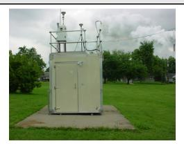
The monitoring site is a stationary equipment shelter located on the grounds of the Watson Lane Elementary School in Louisville, Kentucky. The sample inlets are 4 meters above ground level and 34 meters from the nearest road. Upon inspection, the sample lines and monitors were found to be in good condition. The air monitoring site meets the criteria established by 40 CFR Part 58, Appendices C, D, E and G.
