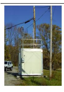
The monitoring site is a stationary equipment shelter located at the intersection of KY 338 and Lower River Road near East Bend, Kentucky. The sample inlet is 15 meters from the nearest road. Upon inspection, the sample line and monitor were found to be in good condition. The site meets the requirements of 40 CFR 58, Appendices C, D and E.
