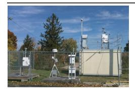
The monitoring site is a stationary equipment shelter located on the grounds of the Fayette County Health Department building in Lexington, Kentucky. The sample inlets are 122 meters from the nearest road. Upon inspection, the sample lines and monitors were found to be in good condition. The site meets the requirements of 40 CFR 58, Appendices A, C, D, E and G.
