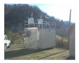
The monitoring site is a stationary equipment shelter located behind the KYTC District Office building in Pikeville, KY. The sample inlets are 88 meters from the nearest road. Upon inspection the sample lines and monitors were found to be in good condition. This site meets the requirements of 40 CFR 58, Appendices A, C, D, E and G.
