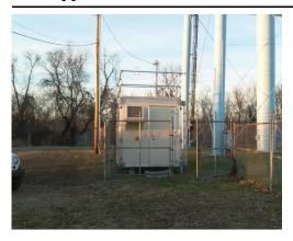
The monitoring site is a stationary equipment shelter located on the grounds of a water tower near the intersection of Scott Street and Center Avenue in Worthington, Kentucky. The sample inlets are 18 meters from the nearest road. Upon inspection, the sample lines and monitors were found to be in good condition. The site meets the requirements of 40 CFR 58, Appendices C, D, E and G.
