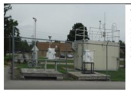
The monitoring site is a stationary equipment shelter located on the grounds of the Fayette County Health Department building in Lexington, Kentucky. The sample inlets are 118 meters from the nearest road. Upon inspection, the sample lines and monitors were found to be in good condition. The site meets the requirements of 40 CFR 58, Appendices A, C, D, E and G.
