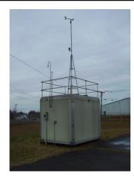
The monitoring site is a stationary equipment shelter located on the grounds of the KYTC Garage on Harding Road (KY1008) in Franklin, Kentucky. The sample inlet is 41.5 meters from the nearest road. Upon inspection, the sample line and monitor were found to be in good condition. The site meets the requirements of 40 CFR 58, Appendices A, C, D, and E.
