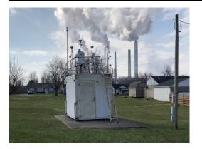
The monitoring site is a stationary equipment shelter located on the grounds of the Watson Lane Elementary School in Louisville, Kentucky. The sample inlets are 4 meters above ground level and 30.3 meters from the nearest road. Upon inspection, the sample lines and monitors were found to be in good condition. The air monitoring site meets the criteria established by 40 CFR Part 58, Appendices C, D, E and G.
