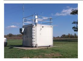
The monitoring site is a stationary equipment shelter located at the residence of 763 Bloodworth Road in Livingston County, Kentucky. The sample inlets are 8 meters from the nearest road, which is an access road for a residence. Upon inspection, the inlet and sampler were found to be in good condition. The site meets the requirements of 40 CFR 58, Appendices A, C, D, and E.
