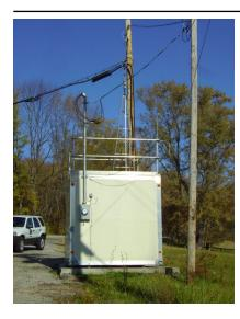
The monitoring site is a stationary equipment shelter located at the intersection of KY 338 and Lower River Road near East Bend, Kentucky. The sample inlet is 15 meters from the nearest road. Upon inspection, the sample line and monitor were found to be in good condition. The site meets the requirements of 40 CFR 58, Appendices A,C, D and E.
