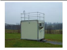
The monitoring site is a stationary equipment shelter located on the grounds of the Kentucky Transportation Cabinet Highway garage in Buckner, Kentucky. The sample inlet is 51 meters from the nearest road. Upon inspection, the sample line and monitor were found to be in good condition. The site meets the requirements of 40 CFR 58, Appendices C, D, and E.
