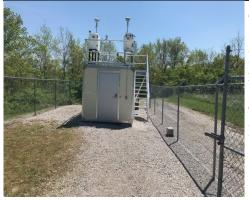
The monitoring site is a stationary equipment shelter located on farmland owned by Northern Kentucky University in Highland Heights, Kentucky. The sample inlets are 448 meters from the nearest road, which is Interstate 275. Upon inspection, the sample lines and monitors were found to be in good condition. The site meets the requirements of 40 CFR 58, Appendices A, C, D, E and G.
