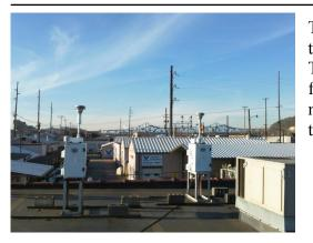
The monitoring site is located on the west end of the roof of the Valvoline Oil complex building in Ashland, Kentucky. The building is one story tall. The sample inlets are 75 meters from the nearest road. Upon inspection, the sample inlets and monitors were found to be in good condition. The site meets the requirements of 40 CFR 58, Appendices A, C, D and E.
