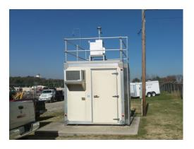
The monitoring site is a stationary equipment shelter located on the grounds of the Somerset Gas Company Warehouse on Clifty Street in Somerset, KY. The sample inlets are 10 meters from the nearest road, which is a dead-end street with little traffic. Upon inspection the sample line and monitors were found to be in good condition. The site meets the requirements of 40 CFR 58, Appendices A, C, D, and E.
