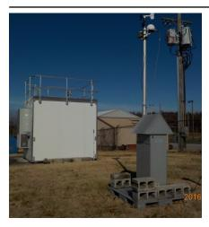
The monitoring site is a stationary equipment shelter located on the grounds of the Livingston County Road Dept. facility in Smithland, Kentucky. The sample inlets are 178.9 meters from the nearest road. Upon inspection, the sample lines and monitors were found to be in good condition. The site meets the requirements of 40 CFR 58, Appendices A, C, D, and E.
