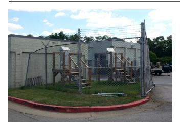
The site is located behind the Gentry Facilities Services building and is adjacent to Eastern Kentucky University's athletic fields. The sample inlets are 2.9 meters from the nearest road. Upon inspection, the sample inlet and monitor were found to be in good condition. The site meets the requirements of 40 CFR 58, Appendices A, C, D and E.
