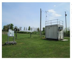
The monitoring site consists of a  $PM_{2.5}$  monitoring platform and an adjacent stationary equipment shelter. The site is located in a field on the property of a private residence, located at 10800 Pilot Rock Road in Hopkinsville, Kentucky. The sample inlets are 116 meters from the nearest road. Upon inspection, the sample inlets and monitors were found to be in good condition. The site meets the requirements of 40 CFR 58, Appendices A, C, D and E.
