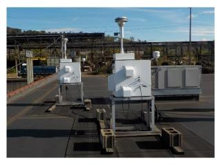
The monitoring site is located on the west end of the roof of the Valvoline Oil complex building in Ashland, Kentucky. The building is one story tall. The sample inlets are 76.6 meters from the nearest road. Upon inspection, the sample inlets and monitors were found to be in good condition. The site meets the requirements of 40 CFR 58, Appendices A, C, D and E.
