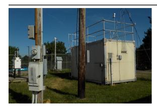
The monitoring site is a stationary equipment shelter located on the grounds of the Fayette County Health Department building in Lexington, Kentucky. The sample inlets are 119 meters from the nearest road. Upon inspection, the sample lines and monitors were found to be in good condition. The site meets the requirements of 40 CFR 58, Appendices A, C, D, E and G.
