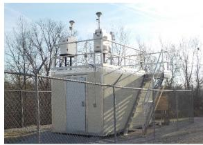
The monitoring site is a stationary equipment shelter located on farmland owned by Northern Kentucky University in Highland Heights, Kentucky. The sample inlets are 451 meters from the nearest road, which is Interstate 275. Upon inspection, the sample lines and monitors were found to be in good condition. The site meets the requirements of 40 CFR 58, Appendices A, C, D, E and G.
