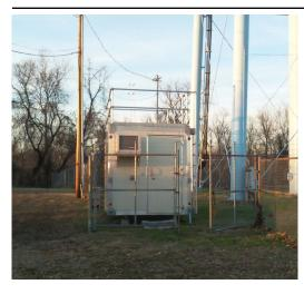
The monitoring site is a stationary equipment shelter located on the grounds of a water tower near the intersection of Scott Street and Center Avenue in Worthington, Kentucky. The sample inlets are 16.6 meters from the nearest road. Upon inspection, the sample lines and monitors were found to be in good condition. The site meets the requirements of 40 CFR 58, Appendices A, C, D, and E.
