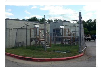
The site is located behind the Gentry Facilities Services building and is adjacent to Eastern Kentucky University's athletic fields. The sample inlets are 3.0 meters from the nearest road. Upon inspection, the sample inlet and monitor were found to be in good condition. The site meets the requirements of 40 CFR 58, Appendices A, C, D and E.
