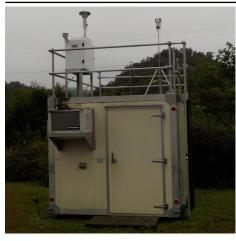
The monitoring site is a stationary equipment shelter located behind the KYTC District Office building in Pikeville, KY. The sample inlets are 91.9 meters from the nearest road. Upon inspection the sample lines and monitors were found to be in good condition. This site meets the requirements of 40 CFR 58, Appendices A, C, D, E and G.
