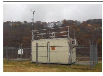
The monitoring site is a stationary equipment shelter located on the grounds of the Perry County Horse Park in Hazard, Kentucky. The sample inlets 29.2 meters from the nearest road. Upon inspection the sample lines and monitors were found to be in good condition. This site meets the requirements of 40 CFR 58, Appendices A, C, D, and E.
