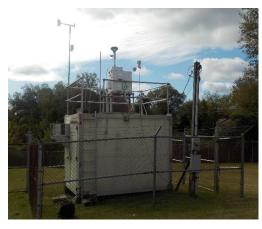
The monitoring site is a stationary equipment shelter located on the grounds of the health department building in Ashland, Kentucky. The sample inlets are 70.7 meters from the nearest road. Upon inspection, the sample lines and monitors were found to be in good condition.
