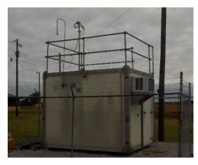
The monitoring site is a stationary equipment shelter located on the athletic fields of the former Lewisport Consolidated Elementary School in Lewisport, Kentucky. The sample inlet is 54.8 meters from the nearest road. Upon inspection, the sample line and monitor were found to be in good condition. The site meets the requirements of 40 CFR 58, Appendices A, C, D, and E.
