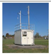
The monitoring site is a stationary equipment shelter located on the grounds of the Kentucky Transportation Cabinet garage in Nicholasville, Kentucky. The sample inlets are 113 meters from the nearest road. Upon inspection, the sample inlets and monitors were found to be in good condition. The site meets the requirements of 40 CFR 58, Appendices A, C, D, and E.
