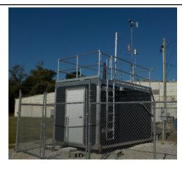
The monitoring site is a stationary equipment shelter located on the grounds behind the Wyndall's Shopping Center in Owensboro, Kentucky. The sample inlets are 45.8 meters from the nearest road. Upon inspection, the sample lines and monitors were found to be in good condition. The site meets the requirements of 40 CFR 58, Appendices A, C, D, E and G.
