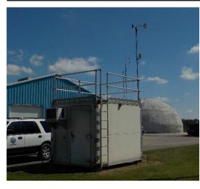
The monitoring site is a stationary equipment shelter located on the grounds of the KYTC Garage on Harding Road (KY1008) in Franklin, Kentucky. The sample inlet is 42.5 meters from the nearest road. Upon inspection, the sample line and monitor were found to be in good condition. The site meets the requirements of 40 CFR 58, Appendices A, C, D, and E.
