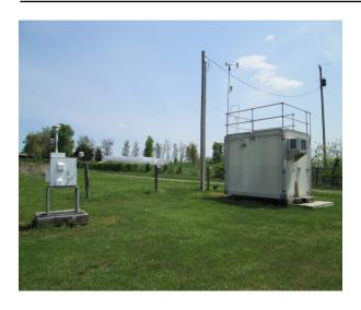
The monitoring site consists of a  $PM_{2.5}$  monitoring platform and an adjacent stationary equipment shelter. The site is located in a field on the property of a private residence, located at 10800 Pilot Rock Road in Hopkinsville, Kentucky. The sample inlets are 116 meters from the nearest road. Upon inspection, the sample inlets and monitors were found to be in good condition. The site meets the requirements of 40 CFR 58, Appendices A, C, D and E.
