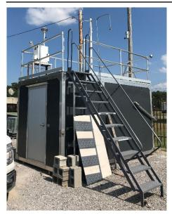
The monitoring site is a stationary equipment shelter located on the grounds of the Jackson Purchase RECC in Paducah, Kentucky. The site meets the requirements established by 40 CFR 58, Appendices C, D, E and G. Due to a new shelter installation in 2018, the sample inlets are now 20.7 meters from the nearest road.
