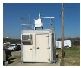
The monitoring site is a stationary equipment shelter located on the grounds of the Somerset Gas Company Warehouse on Clifty Street in Somerset, KY. The sample inlets are 10 meters from the nearest road, which is a dead-end street with little traffic. Upon inspection the sample line and monitors were found to be in good condition. The site meets the requirements of 40 CFR 58, Appendices A, C, D, and E.
