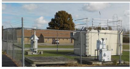
The monitoring site is a stationary equipment shelter located on the grounds of the Fayette County Health Department building in Lexington, Kentucky. The sample inlets are 119 meters from the nearest road. Upon inspection, the sample lines and monitors were found to be in good condition. The site meets the requirements of 40 CFR 58. Appendices A, C, D, E and G.
