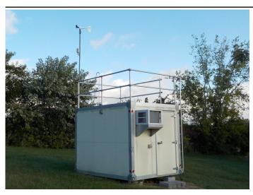
The monitoring site is a stationary equipment shelter located on the grounds of the Kentucky Transportation Cabinet Highway garage in Buckner, Kentucky. The sample inlet is 51 meters from the nearest road. Upon inspection, the sample line and monitor were found to be in good condition. The site meets the requirements of 40 CFR 58, Appendices A, C, D, E, and G.
