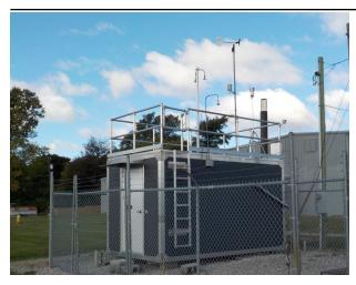
The monitoring site is a stationary equipment shelter located on the grounds behind the Wyndall's Shopping Center in Owensboro, Kentucky. The sample inlets are 45.8 meters from the nearest road. Upon inspection, the sample lines and monitors were found to be in good condition. The site meets the requirements of 40 CFR 58, Appendices A, C, D, and E.
