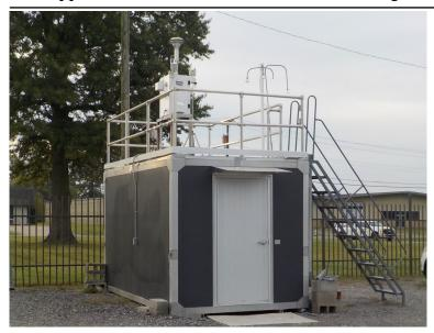
The monitoring site is a stationary equipment shelter located on the former grounds of the Jackson Purchase RECC in Paducah, Kentucky. The sample inlets are 20.7 meters from the nearest road. The site meets the requirements established by 40 CFR 58, Appendices C, D, and E. Due to the current property owners expanding their operations, KDAQ is currently in the process of relocating the site within Paducah, Kentucky.
