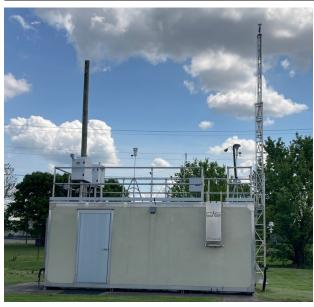
The monitoring site is a stationary equipment shelter located on the grounds of the Firearms Training Center in Louisville, Kentucky. The sample inlet is 4.5 meters above ground level and 53.5 meters from the nearest road. Upon inspection, the sample lines and monitors were found to be in good condition. The air monitoring site meets the criteria established by 40 CFR Part 58, Appendices C, D, E and G.
