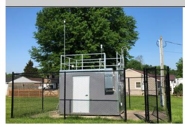
The monitoring site is a stationary equipment shelter located on the grounds of the Watson Lane Elementary School in Louisville, Kentucky. The sample inlets are 4 meters above ground level and 73.7 meters from the nearest road. Upon inspection, the sample lines and monitors were found to be in good condition. The air monitoring site meets the criteria established by 40 CFR Part 58, Appendices C, D, E and G.
