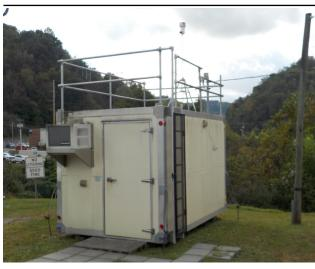
The monitoring site is a stationary equipment shelter located behind the KYTC District Office building in Pikeville, KY. The sample inlets are 91.9 meters from the nearest road. Upon inspection the sample lines and monitors were found to be in good condition. This site meets the requirements of 40 CFR 58, Appendices A, C, D, and E.
