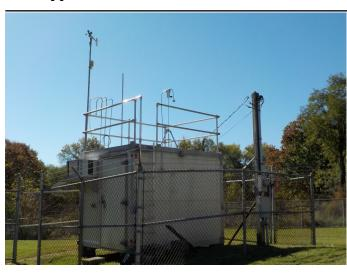
The monitoring site is a stationary equipment shelter located on the grounds of the health department building in Ashland, Kentucky. The sample inlets are 70.7 meters from the nearest road. Upon inspection, the sample lines and monitors were found to be in good condition. The site meets the requirements of 40 CFR 58, Appendices A, C, D, E, and G.
