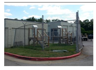
The site is located behind the Gentry Facilities Services building and is adjacent to Eastern Kentucky University's athletic fields. The sample inlets are 3.0 meters from the nearest road. Upon inspection, the sample inlet and monitor were found to be in good condition. The site meets the requirements of 40 CFR 58, Appendices A, C, D and E.
