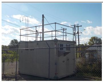
The monitoring site is a stationary equipment shelter located in a fenced-in area near the intersection of Second and Carpenter Streets in Shepherdsville, Kentucky. The sample inlets are 66.4 meters from the nearest road. Upon inspection, the sample lines and monitors were found to be in good condition. The site meets the requirements of 40 CFR 58, Appendices A, C, D, E, and G.
