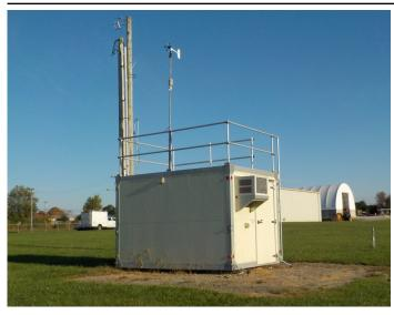
The monitoring site is a stationary equipment shelter located on the grounds of the Kentucky Transportation Cabinet garage in Nicholasville, Kentucky. The sample inlets are 113 meters from the nearest road. Upon inspection, the sample inlets and monitors were found to be in good condition. The site meets the requirements of 40 CFR 58, Appendices A, C, D, E, and G.
