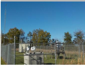
The monitoring site is a stationary equipment shelter in a fenced area located in a remote section of Camp Webb in Grayson, Kentucky. The nearest road is a service road to the site and is 106 meters from the site. Upon inspection, the sample lines and monitors were found to be in good condition. The site meets the requirements of 40 CFR 58, Appendices A, C, D, E, and G.
