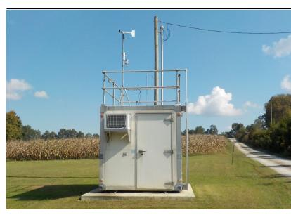
The monitoring site consists of a PM<sub>2.5</sub> monitoring platform and an adjacent stationary equipment shelter. The site is located in a field on the property of a private residence, located at 10800 Pilot Rock Road in Hopkinsville, Kentucky. The sample inlets are 116 meters from the nearest road. Upon inspection, the sample inlets and monitors were found to be in good condition. The site meets the requirements of 40 CFR 58, Appendices A, C, D and E.
