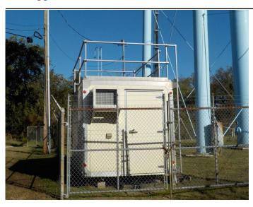
The monitoring site is a stationary equipment shelter located on the grounds of a water tower near the intersection of Scott Street and Center Avenue in Worthington, Kentucky. The sample inlets are 16.6 meters from the nearest road. Upon inspection, the sample lines and monitors were found to be in good condition. The site meets the requirements of 40 CFR 58, Appendices A, C, D, E, and G.
