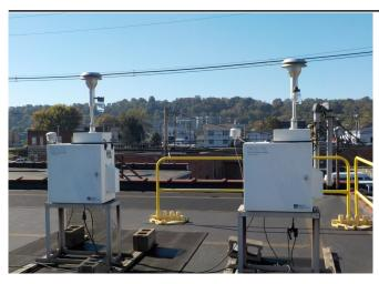
The monitoring site is located on the west end of the roof of the Valvoline Oil complex building in Ashland, Kentucky. The building is one story tall. The sample inlets are 76.6 meters from the nearest road. Upon inspection, the sample inlets and monitors were found to be in good condition. The site meets the requirements of 40 CFR 58, Appendices A, C, D, E, and G.
