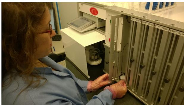
*Environmental technologist Ashley Bedel loads DAQ's Autohandler with  $PM_{2.5}$  filters for weighing. (Photo: DAQ)*
