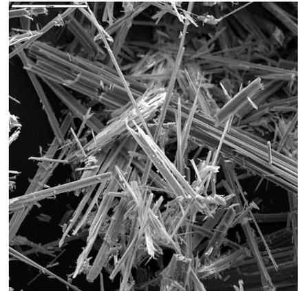
Scanning electron micrograph of anthophyllite asbestos fibers. (Photo: U.S. Geological Survey)
