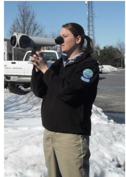
*Field inspector Courtney Shattuck demonstrates the use of a Nasal Ranger, which is used to determine whether an odor exceeds the threshold determined by Kentucky's odor regulation. (Photo: DAQ)*
