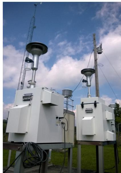
*The particulate matter sampling platform at the Grayson Lake ambient air monitoring station collects PM<sub>2.5</sub> and PM<sub>10</sub> samples. A meteorological tower can be seen in the background. (Photo: DAQ)*
