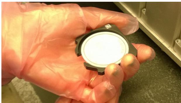
*This  $PM_{2.5}$  filter is weighed before and after air sampling. (Photo: DAQ)*
