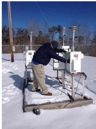
*Environmental scientist Jeff Patton checks one of the air monitors at the Grayson Lake monitoring station. (Photo: DAQ)*
