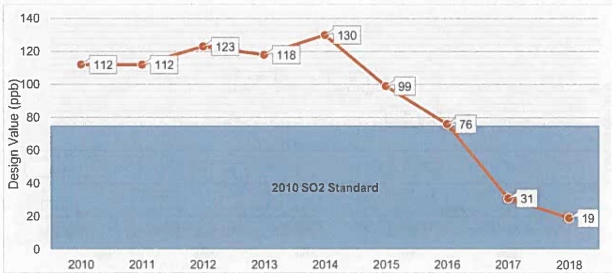
As can be seen from the comparison of the change in the design value at Watson Lane to the change in SO<sub>2</sub> emissions from Mill Creek (figure 4), they are directly correlated.
