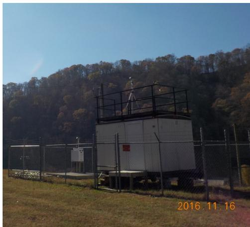
The monitoring site is a stationary equipment shelter located on the grounds of the Perry County Horse Park in Hazard, Kentucky. The sample inlets 29.2 meters from the nearest road. Upon inspection the sample lines and monitors were found to be in good condition. This site meets the requirements of 40 CFR 58, Appendices A, C, D, and E.
