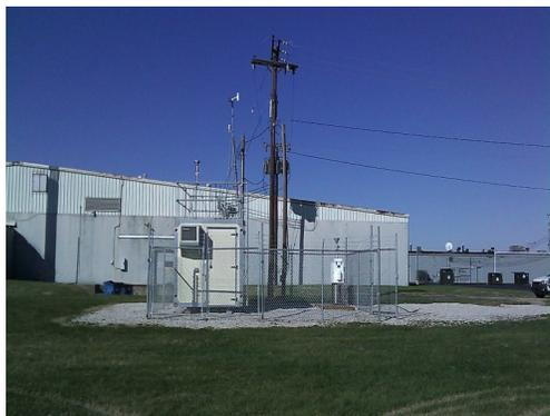
The monitoring site is a stationary equipment shelter located on the grounds behind the Wyndall's Shopping Center in Owensboro, Kentucky. The sample inlets are 48.5 meters from the nearest road. Upon inspection, the sample lines and monitors were found to be in good condition. The site meets the requirements of 40 CFR 58, Appendices A, C, D, E and G.
