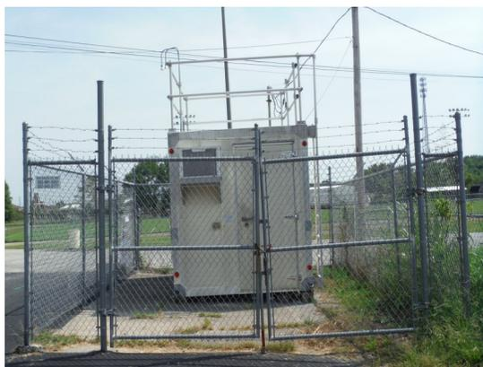
The monitoring site is a stationary equipment shelter located in a fenced-in area near the intersection of Second and Carpenter Streets in Shepherdsville, Kentucky. The sample inlets are 58 meters from the nearest road. Upon inspection, the sample lines and monitors were found to be in good condition. The site meets the requirements of 40 CFR 58, Appendices A, C, D, and E.
