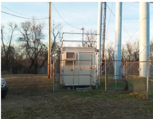
The monitoring site is a stationary equipment shelter located on the grounds of a water tower near the intersection of Scott Street and Center Avenue in Worthington, Kentucky. The sample inlets are 16.2 meters from the nearest road. Upon inspection, the sample lines and monitors were found to be in good condition. The site meets the requirements of 40 CFR 58, Appendices A, C, D, and E.
