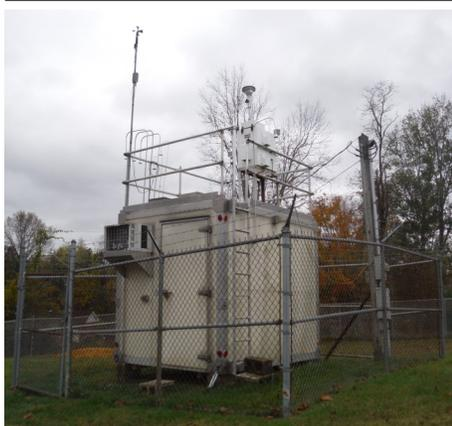
The monitoring site is a stationary equipment shelter located on the grounds of the health department building in Ashland, Kentucky. The sample inlets are 70 meters from the nearest road. Upon inspection, the sample lines and monitors were found to be in good condition.
