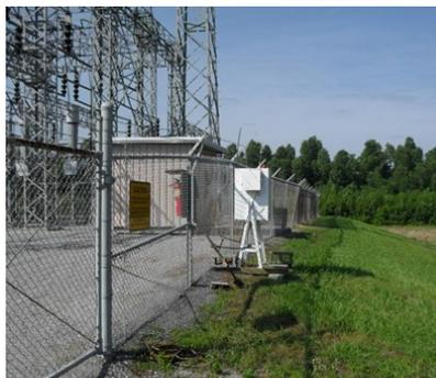
The monitoring site is located off Ballpark Road in Calvert City, Kentucky. The inlets are approximately 231.6 meters from the nearest road. Upon inspection, the sample inlets and monitors were found to be in good condition.
