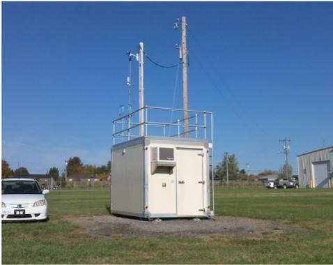
The monitoring site is a stationary equipment shelter located on the grounds of the Kentucky Transportation Cabinet garage in Nicholasville, Kentucky. The sample inlets are 112.3 meters from the nearest road. Upon inspection, the sample inlets and monitors were found to be in good condition. The site meets the requirements of 40 CFR 58, Appendices A, C, D, and E.
