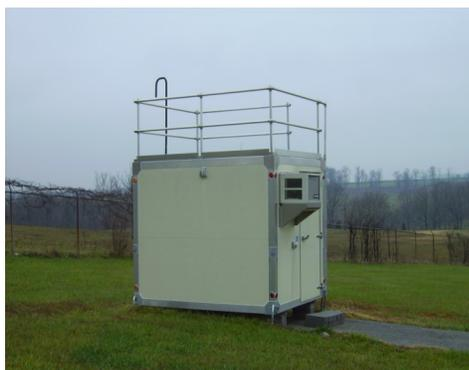
The monitoring site is a stationary equipment shelter located on the grounds of the Kentucky Transportation Cabinet Highway garage in Buckner, Kentucky. The sample inlet is 51 meters from the nearest road. Upon inspection, the sample line and monitor were found to be in good condition. The site meets the requirements of 40 CFR 58, Appendices C, D, and E.
