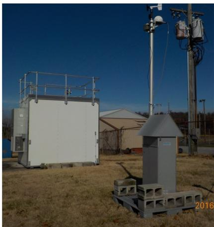
The monitoring site is a stationary equipment shelter located on the grounds of the Livingston County Road Dept. facility in Smithland, Kentucky. The sample inlets are 178.9 meters from the nearest road. Upon inspection, the sample lines and monitors were found to be in good condition. The site meets the requirements of 40 CFR 58, Appendices A, C, D, and E.
