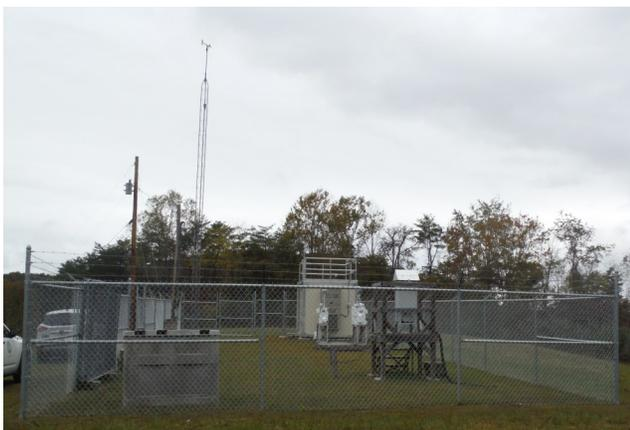
The monitoring site is a stationary equipment shelter in a fenced area located in a remote section of Camp Webb in Grayson, Kentucky. The nearest road is a service road to the site and is 108 meters from the site. Upon inspection, the sample lines and monitors were found to be in good condition. The site meets the requirements of 40 CFR 58, Appendices A, C, D, and E.
