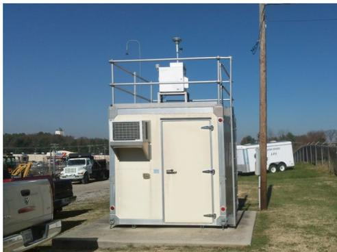
The monitoring site is a stationary equipment shelter located on the grounds of the Somerset Gas Company Warehouse on Clifty Street in Somerset, KY. The sample inlets are 10 meters from the nearest road, which is a dead-end street with little traffic. Upon inspection the sample line and monitors were found to be in good condition. The site meets the requirements of 40 CFR 58, Appendices A, C, D, and E.
