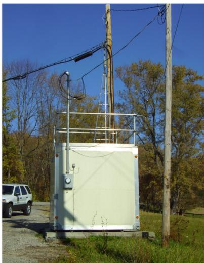
The monitoring site is a stationary equipment shelter located at the intersection of KY 338 and Lower River Road near East Bend, Kentucky. The sample inlet is 15 meters from the nearest road. Upon inspection, the sample line and monitor were found to be in good condition. The site meets the requirements of 40 CFR 58, Appendices A,C, D and E.
