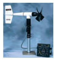
For offshore and marine use, **Model 05106**, **Wind Monitor-MA** features special waterproof bearing lubricant and a sealed, heavy duty cable pigtail in place of the standard junction box. Separate signal conditioning for voltage or current outputs is available.
