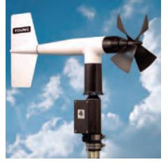
potentiometer housed in a sealed chamber. With a known excitation voltage applied to the potentiometer, the output voltage is directly proportional to vane angle. A mounting orientation ring assures correct realignment of the wind direction reference when the instrument is removed for maintenance.
