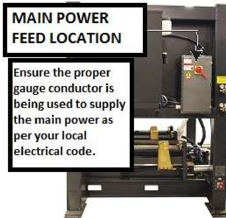
Figure A.4 – Main power feed connection
