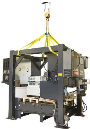
Figure A.1 – Lifting method 1
