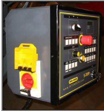
Main Disconnect switch is located on the side on the machine control box.
