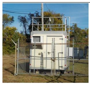
The monitoring site is a stationary equipment shelter located on the grounds of a water tower near the intersection of Scott Street and Center Avenue in Worthington, Kentucky. The sample inlets are 19 meters from the nearest road. Upon inspection, the sample lines and monitors were found to be in good condition. The site meets the requirements of 40 CFR 58, Appendices A, C, D, E, and G.
