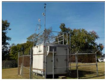
The monitoring site is a stationary equipment shelter located on the grounds of the health department building in Ashland, Kentucky. The sample inlets are 60 meters from the nearest road. Upon inspection, the sample lines and monitors were found to be in good condition. The site meets the requirements of 40 CFR 58, Appendices A, C, D, E, and G.
