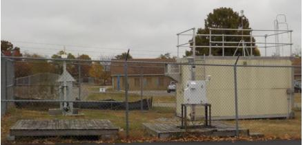
The monitoring site is a stationary equipment shelter located on the grounds of the Fayette County Health Department building in Lexington, Kentucky. The sample inlets are 122 meters from the nearest road. Upon inspection, the sample lines and monitors were found to be in good condition. The site meets the requirements of 40 CFR 58, Appendices A, C, D, E and G.
