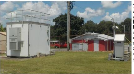
The monitoring site is a stationary equipment shelter located on the grounds of the Livingston County Road Dept. facility in Smithland, Kentucky. The sample inlets are 136 meters from the nearest road. Upon inspection, the sample lines and monitors were found to be in good The site meets condition. the requirements of 40 CFR 58, Appendices A, C, D, and E.
