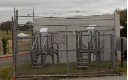
The site is located behind the Gentry Facilities Services building and is adjacent to Eastern Kentucky University's athletic fields. The sample inlets are 3.0 meters from the nearest road. Upon inspection, the sample inlet and monitor were found to be in good condition. The site meets the requirements of 40 CFR 58, Appendices A, C, D and E.
