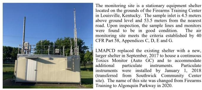
above ground level and 53.5 meters from the nearest road. Upon inspection, the sample lines and monitors were found to be in good condition. The air monitoring site meets the criteria established by 40 CFR Part 58, Appendices C, D, E and G. LMAPCD replaced the existing shelter with a new,
