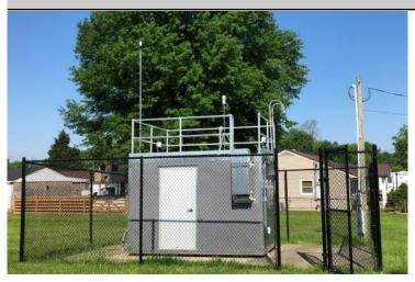
The monitoring site is a stationary equipment shelter located on the grounds of the Watson Lane Elementary School in Louisville, Kentucky. The sample inlets are 4 meters above ground level and 73.7 meters from the nearest road. Upon inspection, the sample lines and monitors were found to be in good condition. The air monitoring site meets the criteria established by 40 CFR Part 58, Appendices C, D, E and G.
