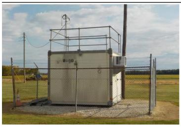
The monitoring site is a stationary equipment shelter located on the athletic fields of the former Lewisport Consolidated Elementary School in Lewisport, Kentucky. The sample inlet is 56 meters from the nearest road. Upon inspection, the sample line and monitor were found to be in good condition. The site meets the requirements of 40 CFR 58, Appendices A,
