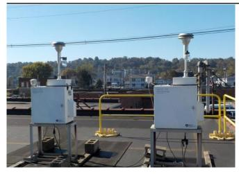
The monitoring site is located on the west end of the roof of the Valvoline Oil complex building in Ashland, Kentucky. The building is one story tall. The sample inlets are 38 meters from the nearest road. Upon inspection, the sample inlets and monitors were found to be in good condition. The site meets the requirements of 40 CFR 58, Appendices A, C, D, and E.
