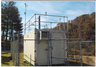
The monitoring site is a stationary equipment shelter located on the grounds of Perry County Park in Hazard, Kentucky. The sample inlets are just over 10 meters from the nearest road and a waiver request for road proximity is included in Appendix L. Otherwise, this site meets the requirements of 40 CFR 58, Appendices A, C, D, E, and G. Beginning in August 2022, Perry County Park became a temporary FEMA site after historic flooding that occurred in July 2022.
