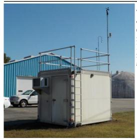
The monitoring site is a stationary equipment shelter located on the grounds of the KYTC Garage on Harding Road (KY1008) in Franklin, Kentucky. The sample inlet is 42.5 meters from the nearest road. Upon inspection, the sample line and monitor were found to be in good condition. The site meets the requirements of 40 CFR 58, Appendices A, C, D, and E.
