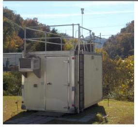
The monitoring site is a stationary equipment shelter located behind the KYTC District Office building in Pikeville, KY. The sample inlets are 96 meters from the nearest road. Upon inspection the sample lines and monitors were found to be in good condition. This site meets the requirements of 40 CFR 58, Appendices A, C, D, and E.
