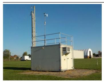
The monitoring site is a stationary equipment shelter located on the grounds of the Kentucky Transportation Cabinet garage in Nicholasville, Kentucky. The sample inlets are 82 meters from the nearest road. Upon inspection, the sample inlets and monitors were found to be in good condition. The site meets the requirements of 40 CFR 58, Appendices A, C, D, E, and G.
