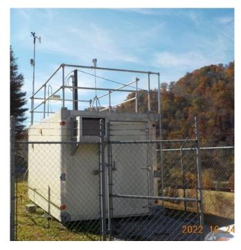
Figure1: Picture of the Hazard air monitoring station.
