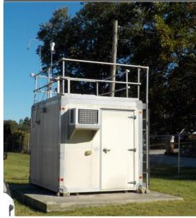
The monitoring site is a stationary equipment shelter located on the grounds of the Somerset Gas Company Warehouse on Clifty Street in Somerset, KY. The site is obstructed by trees and a waiver request for road proximity is included in Appendix L. The trees which are obstructing the site are about to be removed. Otherwise, the site meets the requirements of 40 CFR 58, Appendices A, C, D, E and G.
