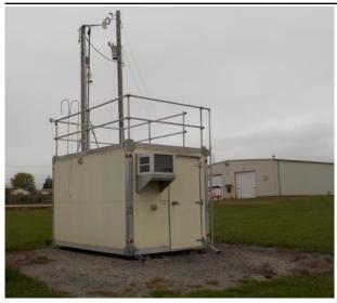
The monitoring site is a stationary equipment shelter located on the grounds of the Kentucky Transportation Cabinet garage in Nicholasville, Kentucky. The sample inlets are 82 meters from the nearest road. Upon inspection, the sample inlets and monitors were found to be in good condition. The site meets the requirements of 40 CFR 58, Appendices A, C, D, E, and G.
