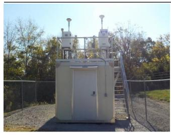
The monitoring site is a stationary equipment shelter located on farmland owned by Northern Kentucky University in Highland Heights, Kentucky. The sample inlets are 450 meters from the nearest road, which is Interstate 275. Upon inspection, the sample lines and monitors were found to be in good condition. The site meets the requirements of 40 CFR 58, Appendices A, C, D, E and G.
