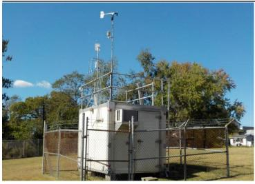
The monitoring site is a stationary equipment shelter located on the grounds of the health department building in Ashland, Kentucky. The sample inlets are 60 meters from the nearest road. Upon inspection, the sample lines and monitors were found to be in good condition. The site meets the requirements of 40 CFR 58, Appendices A, C, D, E, and G.
