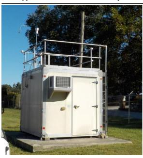
The monitoring site is a stationary equipment shelter located on the grounds of the Somerset Gas Company Warehouse on Clifty Street in Somerset, KY. The site is obstructed by trees and a waiver request for road proximity was included in the 2023 Network Plan and approved by EPA. The trees which are obstructing the site are about to be removed. Otherwise, the site meets the requirements of 40 CFR 58, Appendices A, C, D, E and G.
