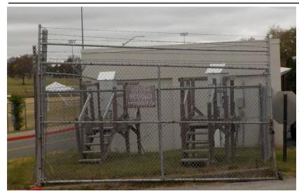
The site is located behind the Gentry Facilities Services building and is adjacent to Eastern Kentucky University's athletic fields. The sample inlets are 3.0 meters from the nearest road. Upon inspection, the sample inlet and monitor were found to be in good condition. The site meets the requirements of 40 CFR 58, Appendices A, C, D and E.
