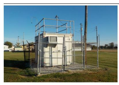
The monitoring site is a stationary equipment shelter located on the athletic fields of the former Lewisport Consolidated Elementary School in Lewisport, Kentucky. The sample inlet is 56 meters from the nearest road. Upon inspection, the sample line and monitor were found to be in good condition. The site meets the requirements of 40 CFR 58, Appendices A, C, D, and E.
