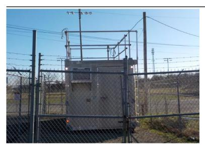
The monitoring site is a stationary equipment shelter located in a fenced-in area near the intersection of Second and Carpenter Streets in Shepherdsville, Kentucky. The sample inlets are 58 meters from the nearest road. Upon inspection, the sample lines and monitors were found to be in good condition. The site meets the requirements of 40 CFR 58, Appendices A, C, D, E, and G.
