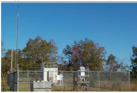
The monitoring site is a stationary equipment shelter in a fenced area located in a remote section of Camp Webb in Grayson, Kentucky. The nearest road is a service road to the site and is 106 meters from the site. Upon inspection, the sample lines and monitors were found to be in good condition. The site meets the requirements of 40 CFR 58, Appendices A, C, D, E, and G.
