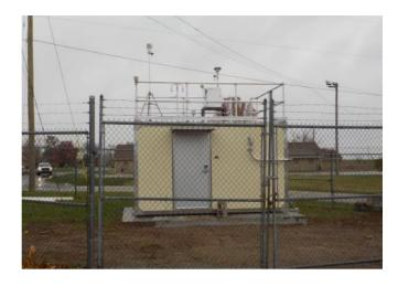
The monitoring site is a stationary equipment shelter located on the grounds of the Fayette County Health Department building in Lexington, Kentucky. The sample inlets are 132 meters from the nearest road. Upon inspection, the sample lines and monitors were found to be in good condition. The site meets the requirements of 40 CFR 58, Appendices A, C, D, E and G.
