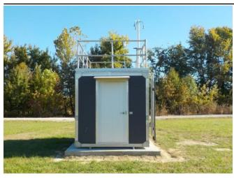
The monitoring site is a stationary equipment shelter located on the grounds of Meadow Lands Elementary School. The sample inlets are 131 meters from the nearest road. The site meets requirements established by 40 CFR 58, Appendices A, C, D, E, and G. This site was previously Owensboro Primary (21-059-0005), which had to be relocated due to land development plans.
