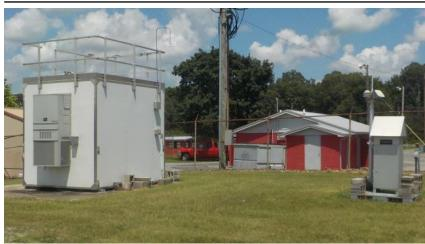
The monitoring site is a stationary equipment shelter located on the grounds of the Livingston County Road Dept. facility in Smithland, Kentucky. The sample inlets are 136 meters from the nearest road. Upon inspection, the sample lines and monitors were found to be in good The site meets condition. the requirements of 40 **CFR** 58, Appendices A, C, D, and E.
