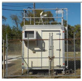
The monitoring site is a stationary equipment shelter located on the grounds of a water tower near the intersection of Scott Street and Center Avenue in Worthington, Kentucky. The sample inlets are 19 meters from the nearest road. Upon inspection, the sample lines and monitors were found to be in good condition. The site meets the requirements of 40 CFR 58, Appendices A, C, D, E, and G.
