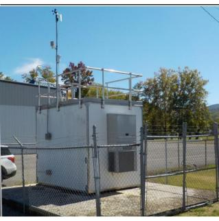
The monitoring site is a stationary equipment shelter located on the grounds of the Middlesboro Airport in Middlesboro, Kentucky. The sample inlets are 96 meters from the nearest road. Upon inspection the sample lines and monitors were found to be in good condition. The site meets the requirements of 40 CFR 58, Appendices A, C, D, E and G.
