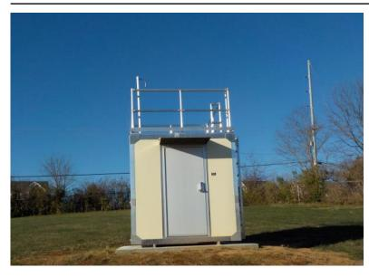
The monitoring site is a stationary equipment shelter located on the grounds of the Kentucky Transportation Cabinet Highway garage in Buckner, Kentucky. The sample inlet is 51 meters from the nearest road. Upon inspection, the sample line and monitor were found to be in good condition. The site meets the requirements of 40 CFR 58, Appendices A, C, D, E, and G.
