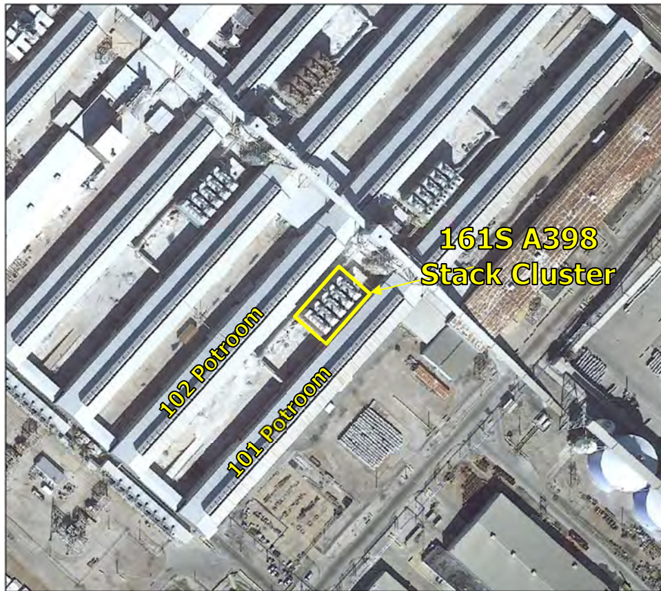
Figure 8. Aerial Image of Potline 1 South A-398 Stack Configuration Showing Close Proximity of Stacks
