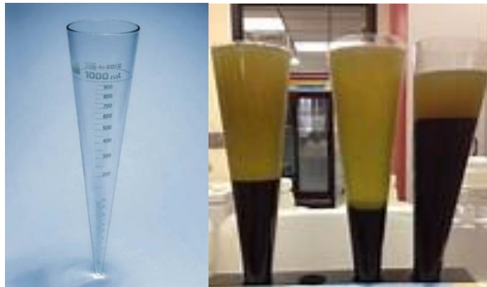
Figure 5.10 Pictures Of An Imhoff Cone Empty And Showing Settleable Solids.
