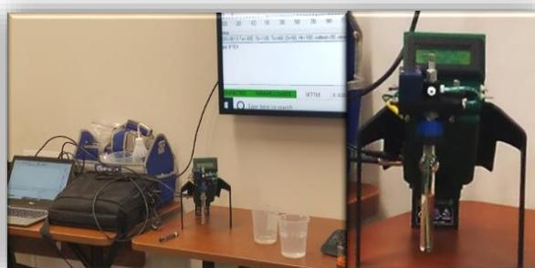
*In June 2018, DWM Field Staff attended training for the FROG 4000 Portable Gas Chromatograph used on-site for groundwater, surface water, vapor intrusion, soil vapor and extraction process monitoring, environmental remediation and site characterization and process monitoring.*
