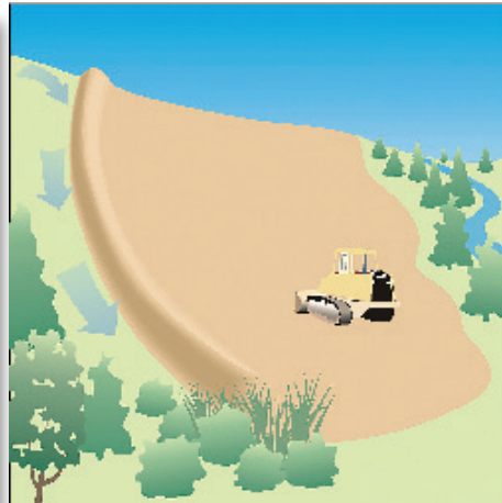
Diversion berms can be temporary or permanent. Make sure they are seeded and mulched immediately after construction. The upslope swale alongside steep berms might need an erosion control blanket to prevent scouring (for drainage system controls, see Section 4.6).
