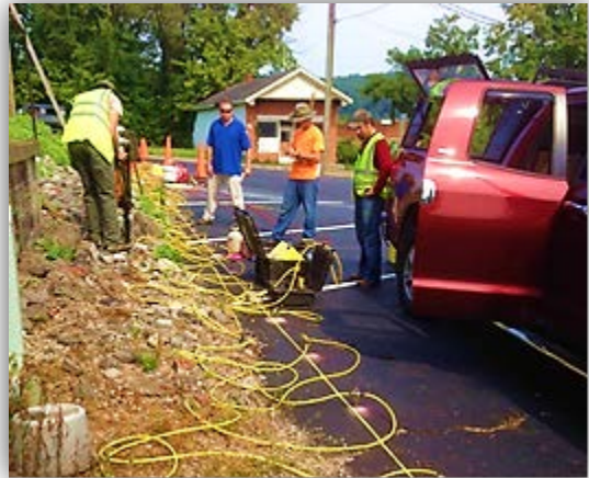
UST Contractors and USTB staff conducting electrical resistivity testing - photo by Brad Highley, August 2015
