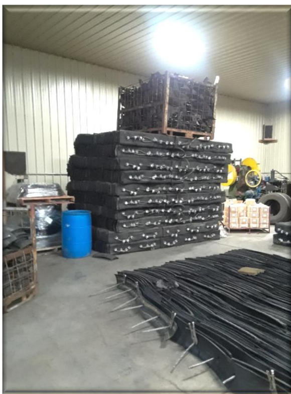
Photo 7: Blasting mats made from recycled tires to contain blast and suppress dust, Bullitt County Photo by Byron J. Bland
