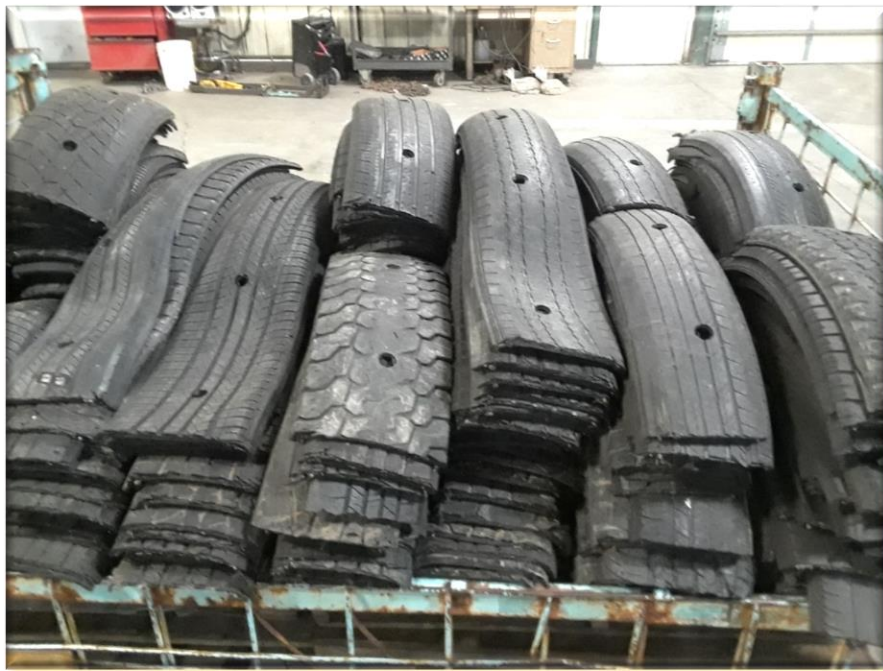
Photo 2: Waste tires used to make blasting mats, Bullitt County Photo by Byron J. Bland
