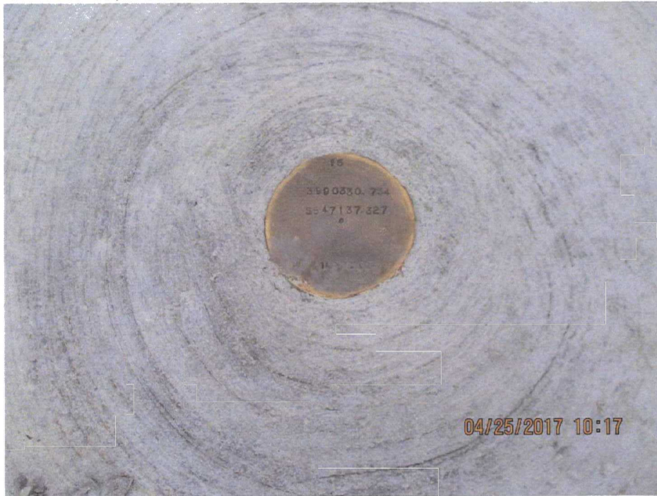
9. Close up of survey monument near the northwest corner of the LF.
