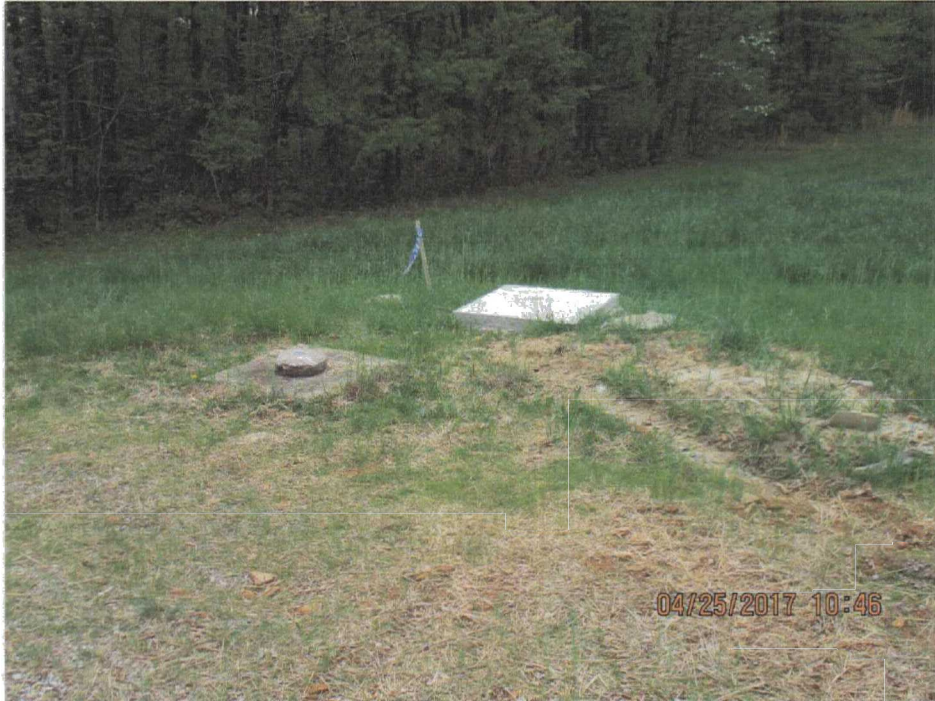
47. Old and new survey markers near the southeastern corner of the LF.
