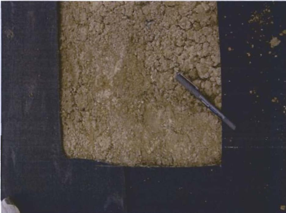
Photo 12: Desiccated Soil Subgrade at LE-1
