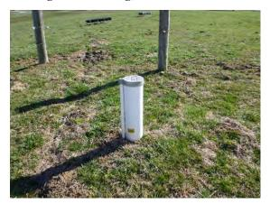
12. If the well is equipped with a vented well cap, check for the presence of the vent screen in the well vent, and clear away any debris that has accumulated on the vent screen. Check the condition of the vent screen to ensure it can prevent insects and animals from entering.
