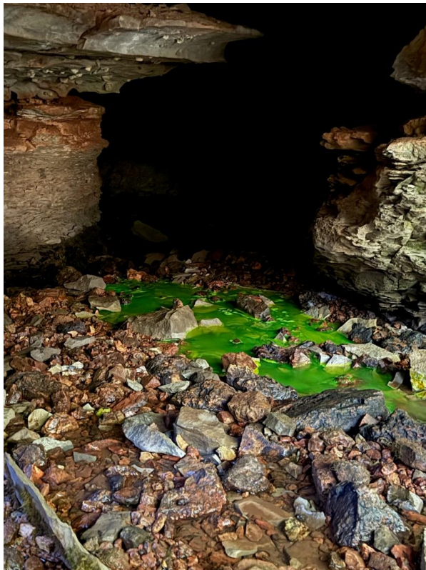
Photo of Uranine Dye Injection
