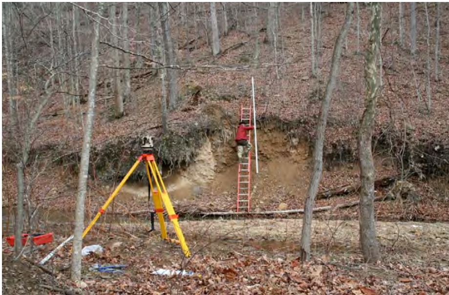
Figure D1: Monitored channel cross-section (SB-0.23a) within 170 ft reach just downstream of SB-0.23 where Sugar Branch erodes colluvium at the base of a steep slope.
