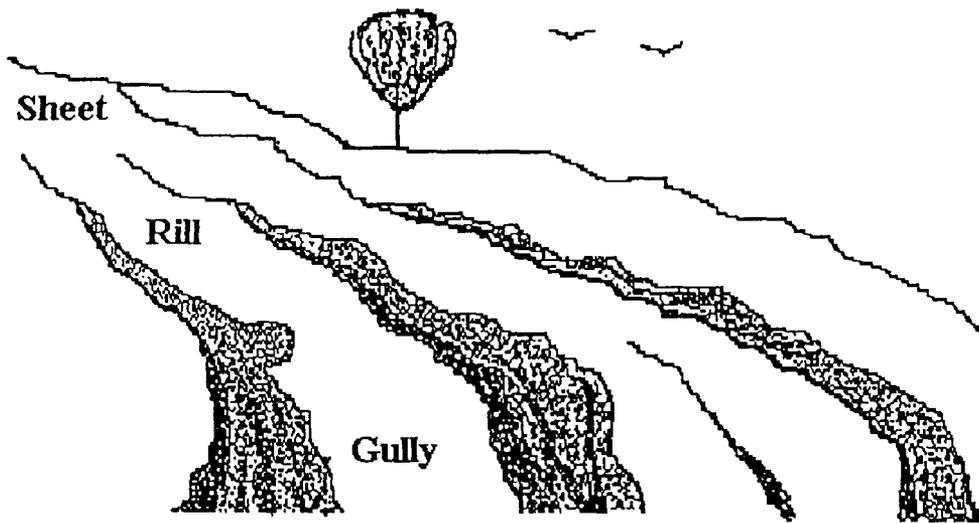
Figure 2. Three types of land-based erosion: sheet, rill, and gully
