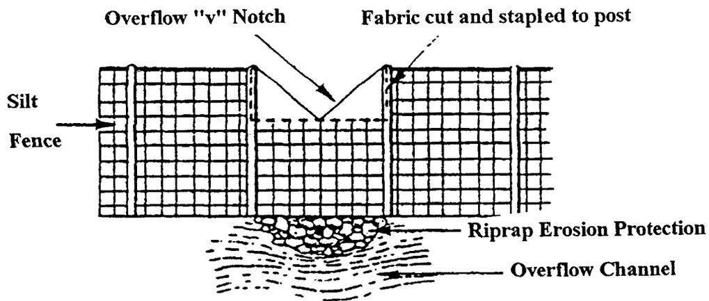
Figure 15. Silt fence weir
