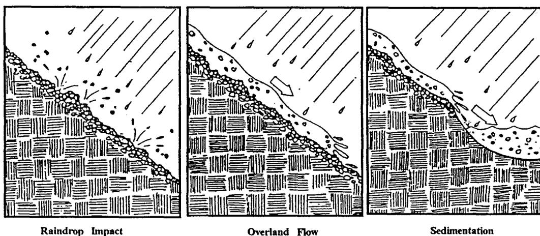
Figure 1. The process of erosion and sedimentation
