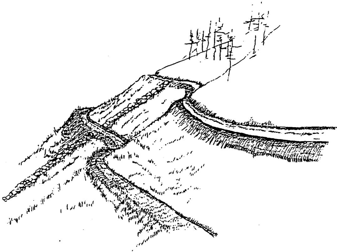
Figure 6. Diversions within the disturbed area reduce slope length and minimize velocity of runoff.
