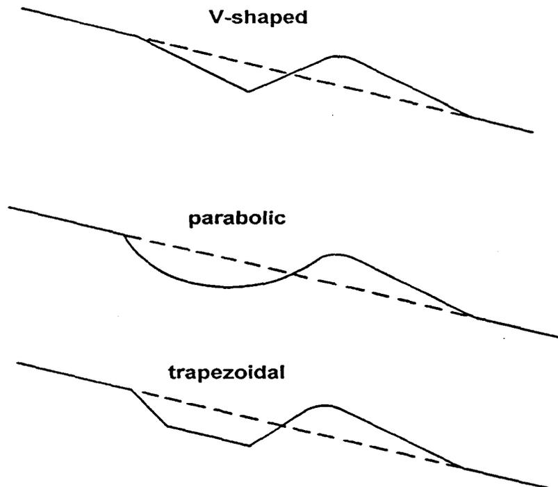
Figure 7. Cross-sectional geometry of diversion ditches.
