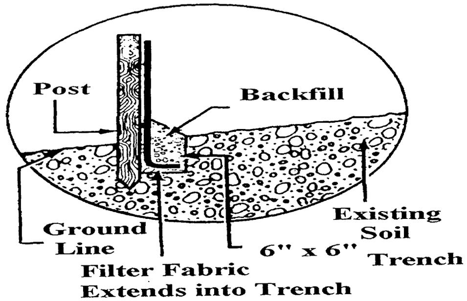
Figure 14. Silt fence installation
