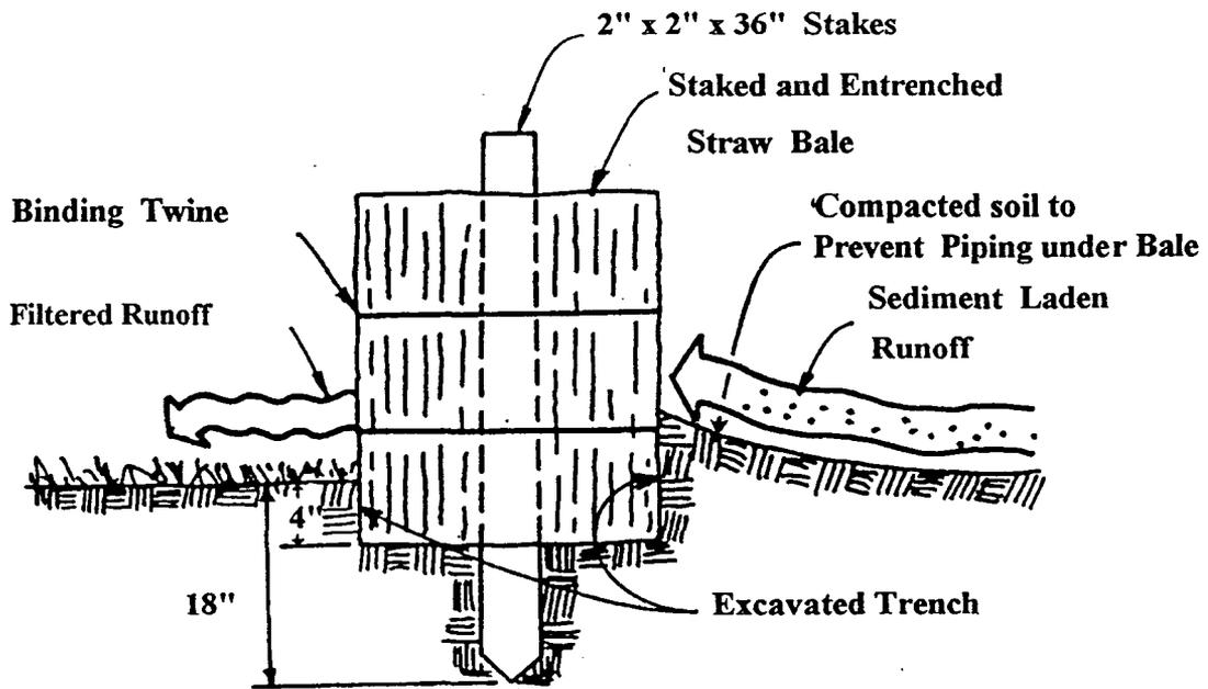
Figure 10. Cross-section of straw bale barrier
