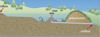
sufficiently to allow excess sediment to settle. Sediment basins shall be designed by a professional engineer licensed in Kentucky.
