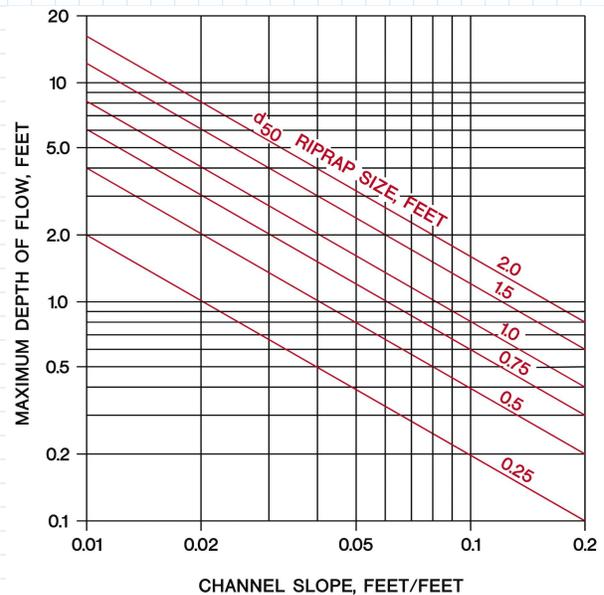
Maximum depth of flow for riprap lined channels
