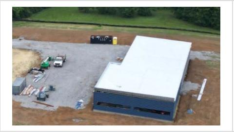
Proper sanitary facility placement: away from inlets, conveyance or surface waters; on level ground; and out of the path of vehicles.
