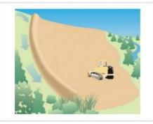
Berms and ditches diverting clean upland runoff around construction sites reduce erosion and sedimentation problems. Seed berms and ditches after construction.
