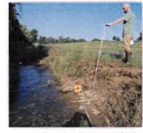
Eroded bank adjacent to (<3' from) Moody Lane. ~3' high, 60°. Notice algae mass on water surface unprotected from sun.
