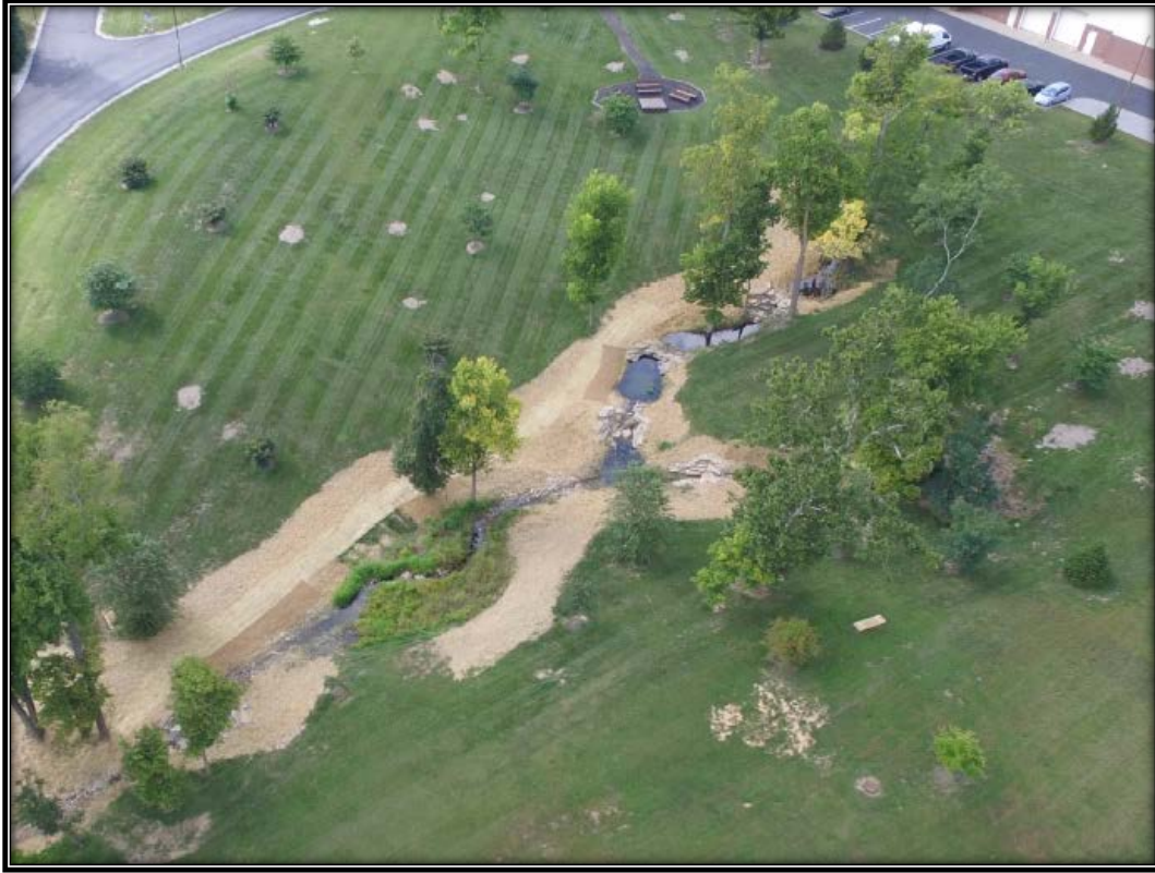
Figure 2.3.2: Gateway College Boone Campus rehabilitated swale
